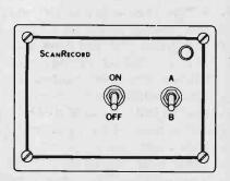
The recorder runs only when a message is received. It does not run when the scanner is just scanning. This lets you record a lot of traffic on one tape. In addition to scanners, it will work with any receiver that has a squelch control.
