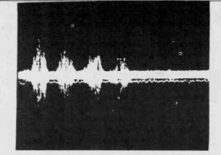
Time exposure (24 sec.) of a triggered (10 Hz) oscilloscope showing a woodpecker frequency in the "dynamic mode" with pulses in each of the four transmitting windows. It uses each window for six seconds.
