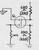
The values of 680 ohms and 100 ohms for the drain and source resistors will be changed to 390 and 220 ohms respectively using 1/4 watt carbon resistors. They are easily located on the main circuit board by their color codes (blue-violet-brown and
