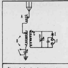
Figure 1. A natural radio receiver. This was an "all-band"communications receiver of yesteryear. It was used for receiving from very long to moderately-short wavelengths back in the 1920's and earlier. This receiver is actually a rather sophisticated design for those days, complete with antena loading coil (a), antenna tuner (b), band changing switch (c), tuning capacitor (d), crystal detector (e), and headphones (f).
