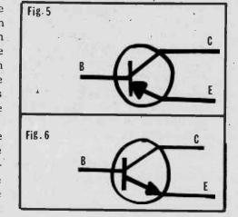
Just remember: the arrow is in the direction of the "positive current flow" for forward bias.
