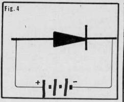
To reverse bias the diode, connect the (+) battery terminal to the N type material and the battery (-) to the P type material (position the diode so that , forward biased, the (+) batthe arrow points toward the (-) battery terminal).
