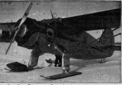
Popular "Norseman" bush plane at Ashuanipi Lake, Feb/48. HF antenna wire was strung from the mast (above the cockpit) to the tail. DF loop antenna may also be seen. In addition, a long trailing antenna wire could be released from the tail for better HF signals, and winched back in before landing.
