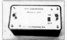
be taken out of line. An internal battery delivers nine volts at only 2 milliamperes, assuring long lifeeven under extended use. An LED signals the converter's "on" status.
