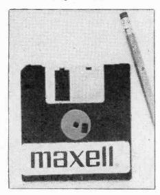
4.As computer sizes scale down so do floppy disks, illustrated here by Maxell's new 3-1/2" entry.
