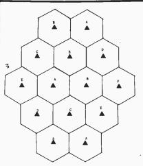
Fig. 1. Cellular radio service areas are often diagrammed using hexagons. Triangles here represent base stations at the center of each cell. Frequency bands assigned to a particular cell are depicted using capital letters. Assignments are so chosen to avoid adjacent cell inteference.
