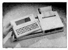
3.The British "Husky," touted as the world's toughest, smallest large-memory (208K) portable computer, shown here with its matching 40-column printer.
