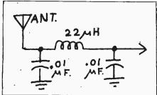
WAVETRAPS: A wavetrap is a tuned circuit designed to reduce the transmission of a narrow swath of frequencies. If it is designed to reduce a wide band of frequencies (while permitting frequencies above and below to pass without attenuation), it is called a stopband filter.
