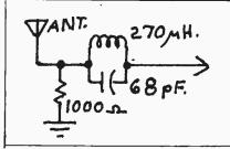
HIGH PASS FILTERS: For shortwave listeners unconcerned with broadcast band or VLF monitoring, the high pass filter is the most commonly used.
