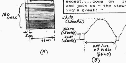
Composition of Slow Scan TV signals, illustrating scan rates and frequencies. Horizontal sweep rate is 15 Hz. Vertical scan takes 8 seconds to produce a single 120 line picture.
