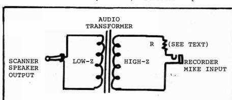
Schematic diagram of recorder coupler
