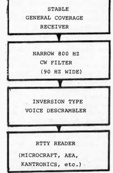
The CW filter selects the discrete channel desired, while inversion-type voice descrambler, commonly available to scanner listeners, is tuned to convert the tones from  $\mathbf{C}\mathbf{W}$ filter sharp (approximately 800 Hz) back to tones near 2 kHz for the RTTY reader or demodulator.
