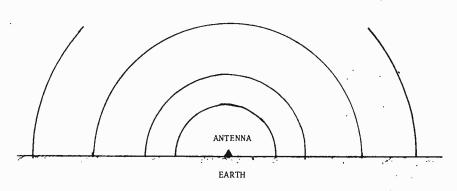
This figure illustrates that as distance from an antenna increases to many wavelengths, the wavefronts change from spherical to planar in shape. In many calculations, considerations are simplified with plane waves. Unfortunately, with terrestrial ELF propagation we are never very many wavelengths away and so have more complex problems.
