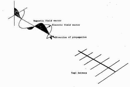
An electromagnetic field consists of two components- an electric field and a magnetic field-- which oscillate in a particular way. If we use an electric field antenna, then for optimum reception the elements must be aligned with the electric field vector.
