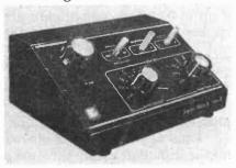
Figure2: A tunable preselector helps frontend shortwave receiver selectivity
