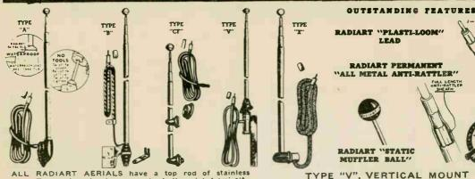
steel. Tubing is extra heavy grade Antimonial Admiralty Brass with a non-peeling plating of copper, then nickel and finally a heavy plating of chromium.
