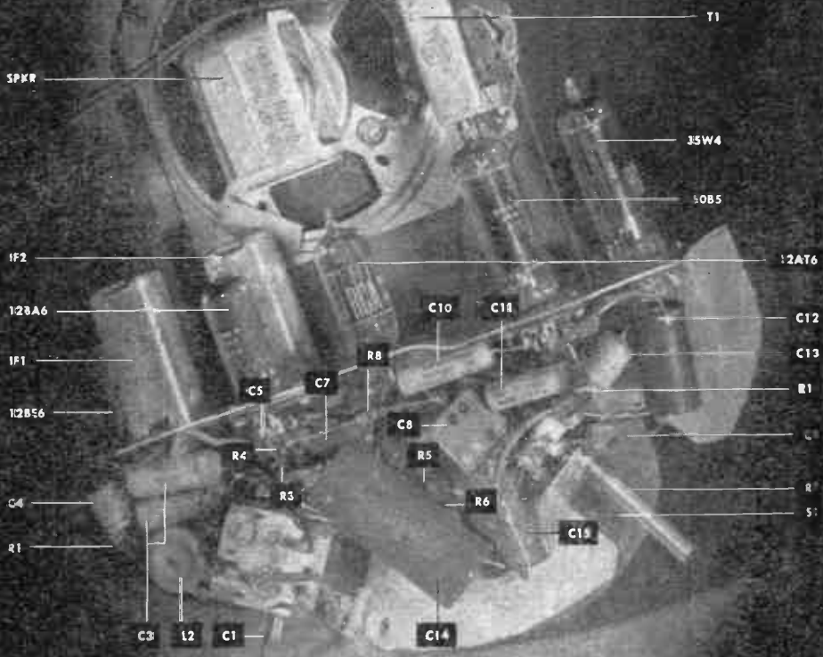
Parts layout must be planned before work begins if the set is to fit snugly in a skillet.
