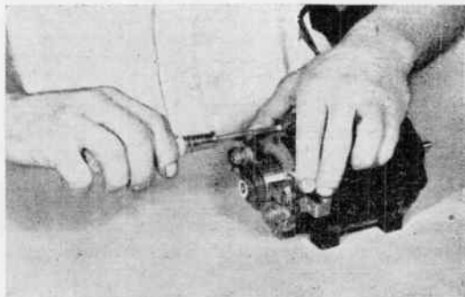
Both brushes must be in perfect alignment on the motor. Their position can be adjusted by loosening two machine screws and then moving the plastic ring
