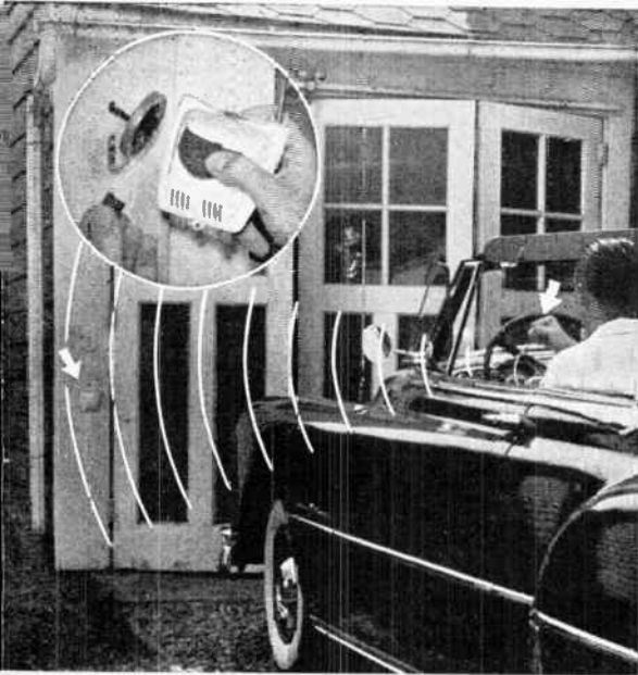
Automatic garage doors can be honked open with this sound-operated switch. Mike is cushioned on rubber, enclosed in a watertight hood.
