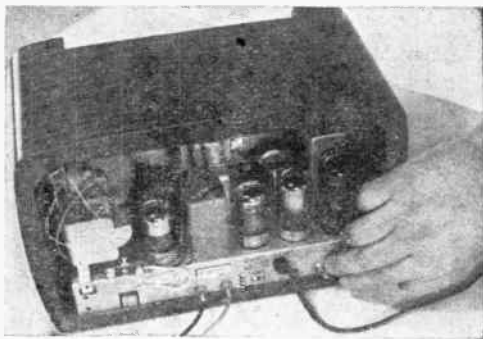
Two jacks and a toggle switch, installed on the chassis of a table radio as shown above, permit the small set to be connected to the speaker of a console model by wires leading from the jacks
