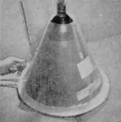
13 The entire metal shell of the 16AP4 is "hot," so it's wise to cover it with a plastic insulating hood and ring. The brackets I bought had a metal ring support.
