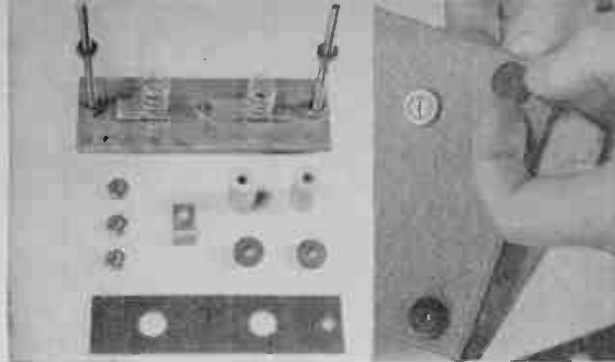
Stiff fiber strips, left, are spaced out on two long 8-32 screws to hold D-size cells that are charged. Right, cushioned feet hold the cabinet.
