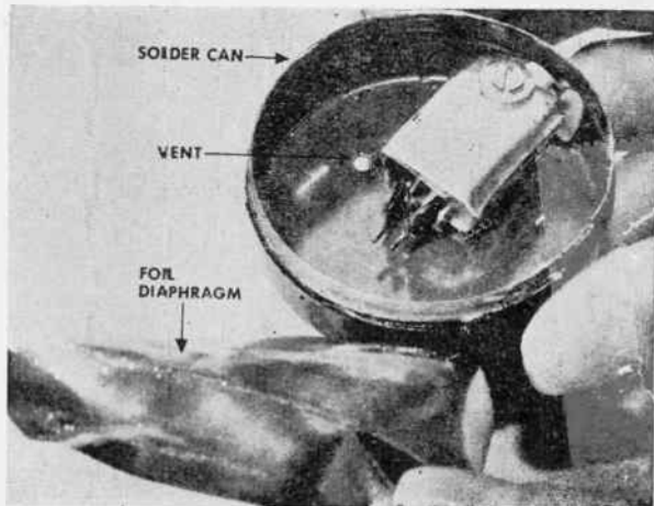
Drilling out rivets permits shell and crystal to be disassembled. The shell is cut down and a wire lever is cemented to the crystal.
