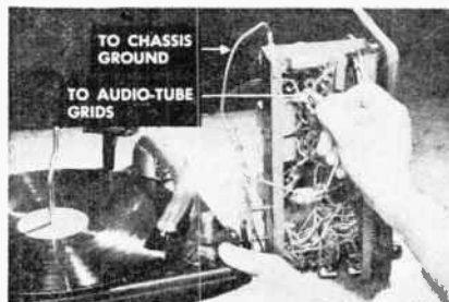
Checking the audio circuits
