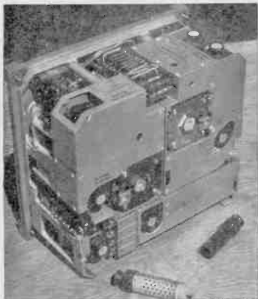
Above is a German superheterodyne tank receiver. It has a range of 27.2 to 33.4 megacycles, and uses a dynamotor that draws 4 amps. from a 12-volt battery
