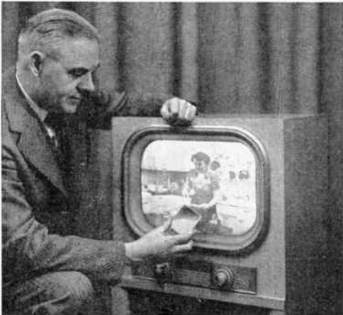
Most annoying lighting trouble is reflection of bright lamps in the viewing screen. An easy test for this is to turn on the lamps and move a hand mirror around on the safety glass.
