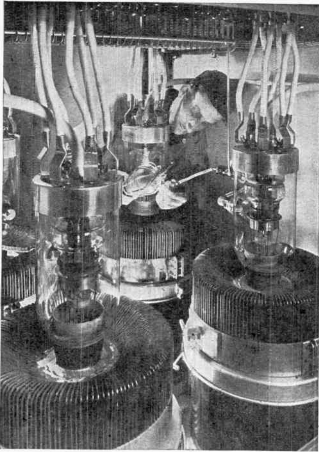
Each of these air-cooled modulator tubes has a 50,000-watt output
