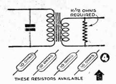
A RADIO engineer, needing a 16<sup>1</sup>/<sub>2</sub>-ohm resistance across an amplifier transformer for testing purposes, found he had nothing but four 10-ohm resistors in his parts drawer, which therefore had to serve. How did he connect them?
