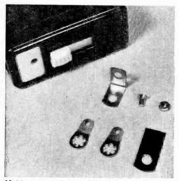
Making a switch out of the slide top of a cigarette case calls for a %" angle bracket, a flat mending plate, soldering lugs, and hardware.
