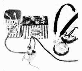
For test purposes standard 1½ and 22½-volt batteries were used, but a penlight cell and a miniature B battery would provide a power supply hardly larger than the radio itself.
