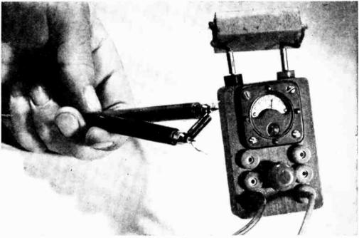
With external battery the pocket-size tester measures two ranges of resistance. Three pen-
