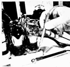
2. Test-point adapter, easily made from wafer tube socket, allows you to check voltages at the tube instead of turning classis over.
