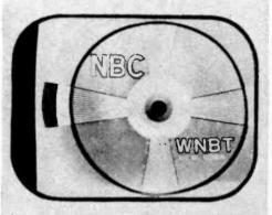
Horizontal centering, like the vertical, brings the picture frame inside the limits of the mask. Misadjustment of this control could also push the picture to the left. Usually a rear adjustment.
