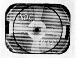
Sound bars break up a picture as shown. They are particularly common on sets using the same intermediate-frequency circuit for sound and picture. Fine-tuning adjustment clears it up.
