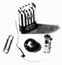
A few of the tiny components. Note the small condenser, volume control, tube, and battery.
