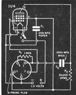
The small parts used can be soldered directly to the 5-prong mounting plug and the 7-pin miniature wafer socket that holds the tube.
