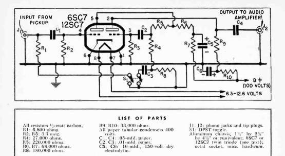
if your set doesn't provide for such a connection, bring the lead from C4 to the "hot" side of the volume control (the outside lug that is not grounded) and connect the shielded lead to the chassis of the radio. A SPST switch in series with the ungrounded lead will enable you to cut out the preamp when listening to the radio.
