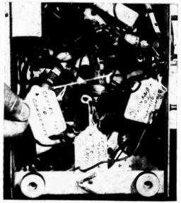
CONSIDERABLE time may be saved and possible errors eliminated by using price tags to mark the wires when making replacement of radio parts. During reassembly, the tags will show exactly where each wire goes. By erasing the pencil marks, the tags may be used many times. Such tags are available at office supply stores.
