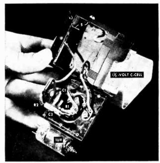
**Layout and wiring** of the parts is simple. The thing to watch for is clearance of the tube and socket in the  $2^{n}$ -wide opening in the case.
