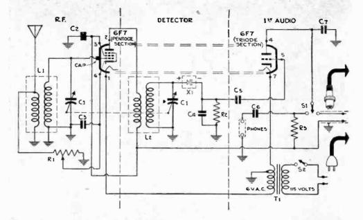
The cathode-regenerative circuit employed in this one-tube tuner is free of whistles and howls, and causes na interference with other radios. A tiny new crystal used in wartime radar equipment acts as the detector, replacing the mare conventional diode.
