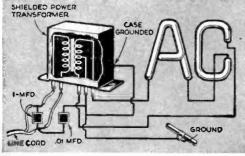
with some sort of built-in filter. Simple remedies can be effected by the amateur serviceman. Those described below call for noise filters put into the appliance circuit itself and will prove highly efficient.
