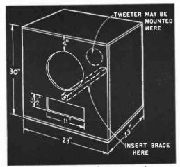
6. A bass-reflex cabinet for a 12" speaker may be made to these dimensions. Use %" plywood.
