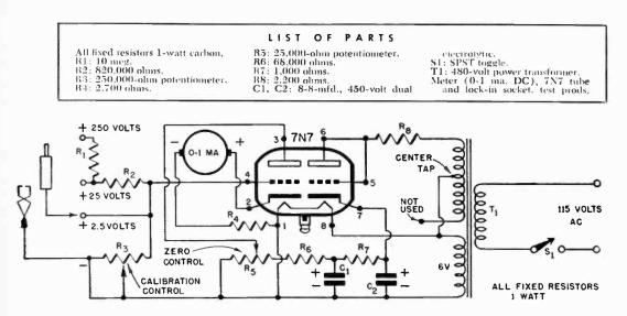
14. Half of the dual triode serves as a power rectifier, the other half as the meter tube, 134
