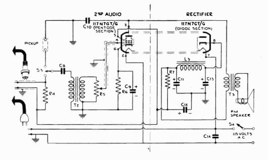
One stage of amplification is enough to drive a 12" speaker at comfortable volume, but a smaller unit can be used if preferred. When operating with a phonograph, the amplifier gives best results if caupled to a crystal pickup of the high-output type.
