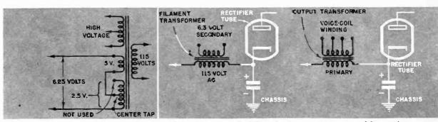
7. Old transformers for 2.5 and 5-volt tubes can be used in modern circuits with 6.3-volt heaters. This arrangement gives 6.25 volts.
