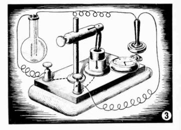
granules in a quiet room. Note, too, how they react to different letters in the alphabet. Such a mike is erratic at various frequencies and is hardly of high fidelity. Held in different positions, it varies in sensitivity, and frequently its granules pack. But in spite of drawbacks, the carbon mike has reached a good stage of development in telephones, walkie-talkies, and tank and plane radios.
