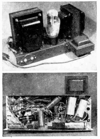
In the rear view of the power pack, the transformer is at left and the two chokes at right, the second being the one on the side. Wiring is shown in the view from the bottom.
