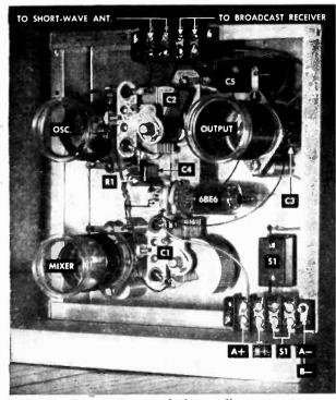
**Coil sockets** and the oscillator capacitor are raised from the chassis by insulated spacers. Solder all leads that go beneath these parts before you actually fasten them into position.
