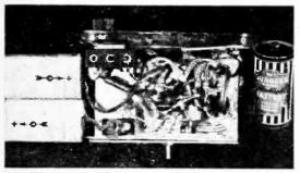
Wiring shouldn't be difficult. Just don't let it spread out. Batteries fit under the chassis. 222
