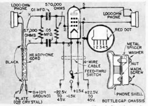
**Tabe connections** are soldered directly to the pins. Use a small iron and try to solder each joint quickly; too much heat may cause damage.
