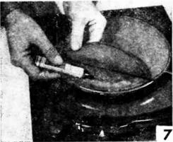
To eliminate mechanically caused hum, vibrations transmitted from the motor to the record must be damped somewhere along the line of travel. A piece of heavy felt glued to the turntable may help.
