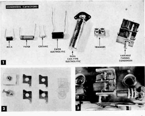
battery-operated receivers a condenser rated at 400 volts allows a safe margin. You might get by with these even in an AC set or amplifier that delivers 250 to 350 volts of B plus, but a few pennies more can buy greater safety in the form of 600-volt condensers. Sometimes heat generated by tubes may melt the wax in which a condenser is sealed. Where this seems likely, try to get capacitors sealed in plastic.
