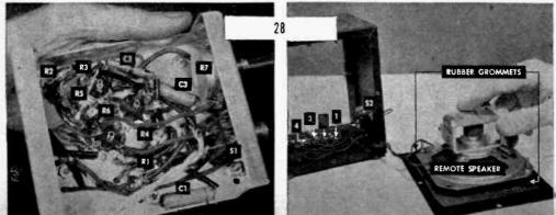
contact terminal strip housed in a 4" by 5" by 6" metal box. Stack a couple of rubber grommets or washers on the screws that hold the speaker to space it back of the panel.
