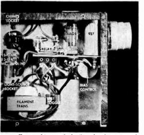
For a cabinet, a 2" by 7" radio chassis is used. The 6-volt transformer and sockets for chimes and light source are fastened to it; other parts are on a separate subchassis.
