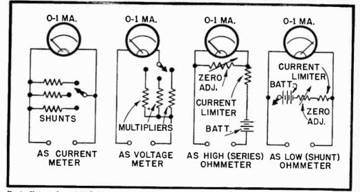
Basic Principles of V-O-M meters. Any fairly sensitive current meter will register higher values of current as well as volts and oluns if
