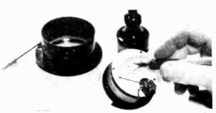
**4.** If a meter is altered to read 0-1 ma, by removing a shunt, the scale must be re-marked.
