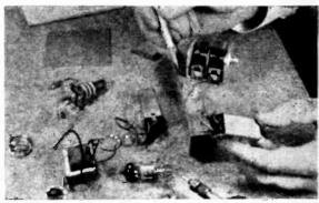
Make trial layouts of the chassis-mounted components before you drill all of the mounting holes. The chassis area is only 2%" by 5".
