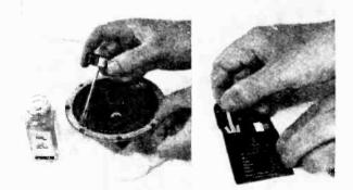
Loosen the cement at the rim Paper centering shims of of the frame to remove a cone different thicknesses can be that has no centering screw obtained in a small kit
