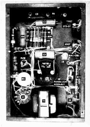
3. A combined classis and cabinet is used for assembling the parts. Layout isn't very critical.
