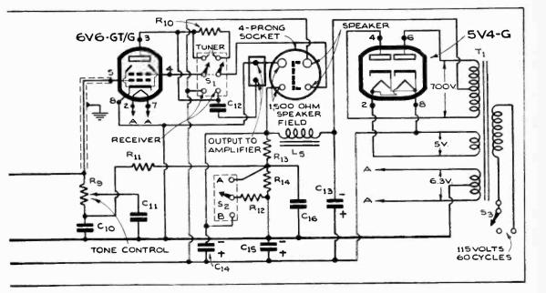
plifier, reverse the positions of both S1 and S2 and replace the speaker plug with the jumper described above. Run a singleconductor cable with a braided external shield from the binding posts to the input connections of the amplifier. The braided shield of the cable, of course, goes to the grounded terminals at tuner and amplifier.
