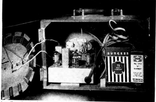
A small wooden cleat behind the chassis keeps it from sliding back in the cabinet. Cleats are
