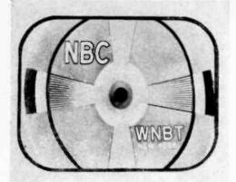
**Height control** is misadjusted. Notice the elongated circle showing that the picture is stretched out vertically. The adjustment is one of the "fixed controls" at the back of set.
