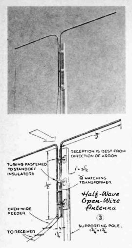
close to a broadcasting station you'll find the easily constructed half-wave dipole efficient.
