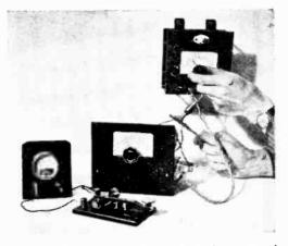
An alternative antenna-tuning methad consists of connecting o laop of wire to a neon or Christmostree bulb, and holding the loop near either end of the plate coil. Energy in the coil lights the bulb.
