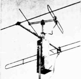
Motor-driven antenna is governed by a switch located at the receiver. A three-wire cable brings power to the roof; the rest of the mechanism is scaled inside a weathertight box.
