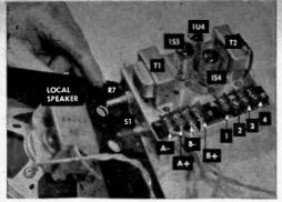
Local station is assembled on a 3%" by 4%" chassis; transformers, tubes, and terminal strips go on top. Controls are on front edge.
