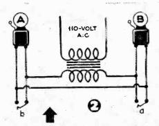
WISHING to save wire, Jones hooked up two bells this way. Button a was to ring bell A, and button b bell B. Although pushing both buttons at once would cause a short circuit. Jones thought this would be of too short duration to harm the transformer, and he expected no trouble. He had trouble anyway. Why?
