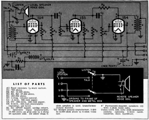
When planning parts layout leave space for batteries; they go in cabinet with amplifier.
