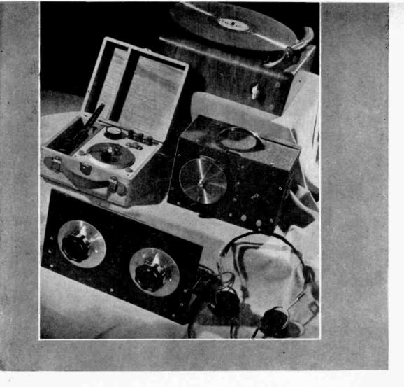
Radio-phonograph combinations strike a new note in crystal-set construction. The complete yet extremely simple unit shown at the right depends upon two relatively recent developments. First is a highoutput pickup that can operate headphones directly without amplification; the second is a preset, fixedcrystal detector. Because this crystal requires no manual adjustment of its cat's whisker, the entire radio can be tucked out of sight inside the cabinet.
