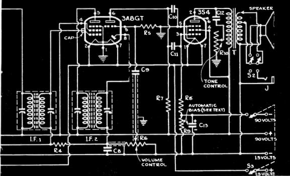
selected because it has room for a 1,000-hour power supply. Battery packs that deliver 1.5 volts for the filaments and 90 volts for the plates are now available in a variety of sizes and shapes. Where portability is a factor, a small pack may be used, in which case the cabinet can be much reduced in size. The larger of the so-called "farm" packs are estimated to be good for a full year of service with this lowdrain circuit, based on average daily use of about three hours.
