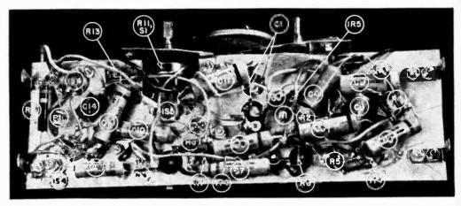
Most of the wiring is done below the chassis. Use the new tiny resistors and condensers to save space.
