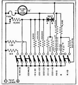
Pushbutton selector switches or individual toggles are used here to simplify switching.
