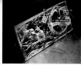
Aluminum foil stapled to the front panel acts as a common ground or chassis and also provides shielding for the variable condenser.
