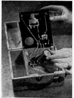
Two separate tuned circuits enable this receiver to distinguish between two or more powerful signals. The alligator clip is used to centertap the antenna coil, L1, when a long aerial is available.
