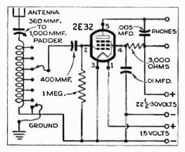
Resistors are ¼ watt, and the tubular condensers 200 volts; phone impedance should be 2,000 chms.
