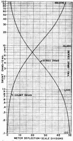
A graph of this type will help you interpret nonlinear shunt and series ohnmeter readings. It should hold for meters built like the one above, or it can be plotted from known values.
