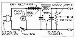
Output of this power supply is variable from 70 to 140 volts. If the ripple is abjectionable, increase the size of the first condenser to 40 mfd.
