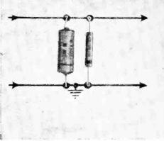
If turning the volume control low produces a "loss of bass" in your receiver, inserting a condenser between volume-control tap and ground may give the failing low notes a boost.
