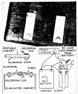
**Contact strips** are added to the bottom of the radio. These must line up with the contacts on the eliminator. The outer one is metative.
