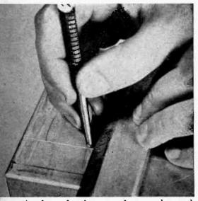
A ruler and a sharp punch are used to mark a chassis. For experimental layouts that may have to be erased, use soft or colored pencil.
