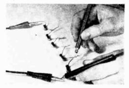
Approximate values of resistors can be determined as at B. By comparing the meter deflection after a timed wait when the condenser is shunted across an unknown resistor with that obtained from a known one, you can gauge the unknown value.
