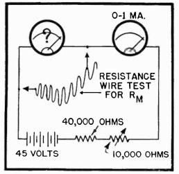
The internal resistance of a meter movement and the current required for full-scale deflection can be determined with this setup.
