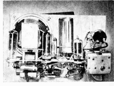
The chassis is a sheet of aluminum bent to the shape of a long. "L." Most of the parts are attached to the projecting leage.
