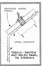
The chassis is a 6" by 6" metal sheet bent to conform with the slope of the wood panel. The cabinet is covered with artificial leather both inside and out.
