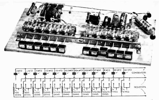
Push-Button Selector Keeps Range of Test Values Handy on Bench
