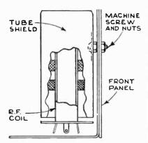
To prevent oscillation and distortion due to stray coupling, the RF coil must be shielded. A suggested method for isolating the coil is to enclose it in an old tube shield which is attached to the chassis as shown above.
