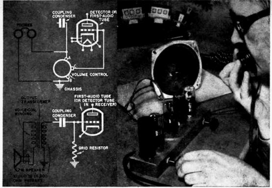
1. Headphones or even a loudspeaker will often replace a crystal microphone. Drawings at the left show connection to common radio circuits. Above, phone is used to test amplifier.
