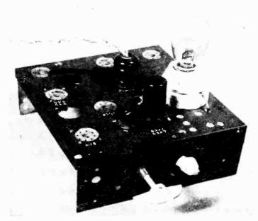
Extro sockets can be added. This chassis has one for testing 6SQ7's
