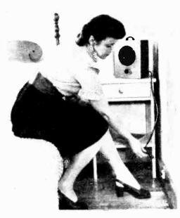
**PIPED PROGRAMS**. You can listen to your console radio in any room in the house with the remote pickup and control system shown below. A portable speaker, plugged into the circuit wherever convenient, has a volume control and an on-off switch that controls the radio,
