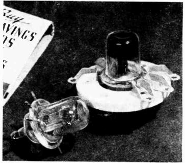
Shawn full size, these tiny acarn triodes wark at 500,000,000 cycles and more. In the socket is a 6-volt tube; the other is a  $1^{1/2}$ -volt type.
