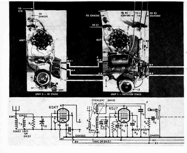
the primary winding of the RF coil. By induction the coil transfers them to the secondary winding where the tuning condenser (in parallel with this part of the coil) selects one particular signal from the jumble.
