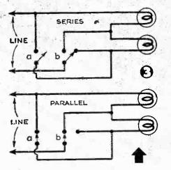
NOT having a double-pole, double-throw switch on hand, a photographer connected a S.P.S.T. switch a and a S.P.D.T. switch b as above to throw two flood lamps from series to parallel or vice versa. As all worked well in the positions shown, he considered himself lucky. Why was he even luckier than he thought?
