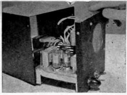
Front panel of metal box is cut for speaker and control shafts; the back cover is removed and replaced with a piece of wire screening.
