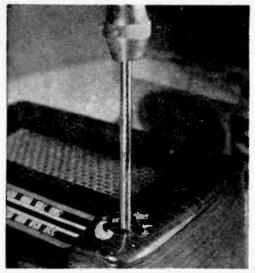
An opening for the indicator tube is made with an expansive bit. For the 6AL7-GT it should be %"; most other tubes need a 1 3/16" hole.
