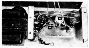
**13.** Remaining parts are wired underneath the chassis, which is then placed in the cabinet.
