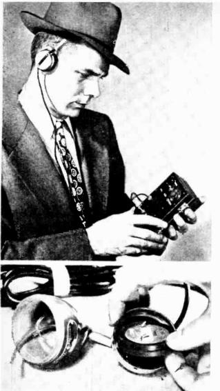
A crystal cartridge, together with its rubber cushion, is removed from a microphone housing.
