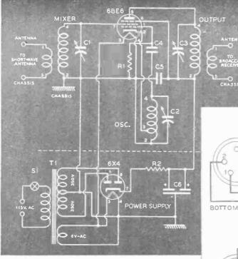
signal is so long as it is steady enough so that you can use it to peak the converter. With a fiber wand, carefully rotate the midget capacitor C3 until the signal reaches maximum strength. Now rotate the mixer control, C1, until the test signal is again brought to maximum. The ground lug adjacent to the antenna input terminal should now be touched to the chassis to see whether this increases volume; if it does, make a permanent connection.
