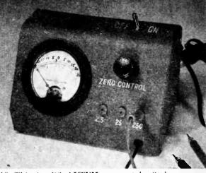
**10.** This simplified VTVM uses one tube. Scale divisions, from 0 to 25, are marked on glass.
