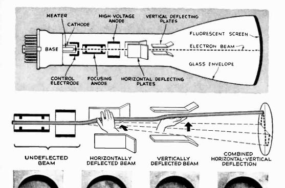
are simultaneously applied to both pairs of plates, so that as the spot moves across the screen it also moves up and down, then the electron beam will trace out a visible pattern (Fig. 4) representing the relationship of the two voltages applied.
