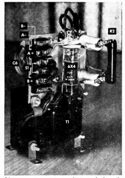
If a separate power supply is used, the only connections to the receiver will be those for antenna and ground. Alternatively, plate and filament voltages can be tapped off an AC set.
