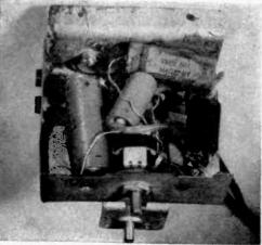
be necessary, depending on the parts you can obtain. One 9002 tube is used as an A.F. amplifier: another, with its plate and grid tied together, serves as a diode half-wave rectifier for the power supply. The third tube, a 9003, acts as detector and R.F. amplifier. Regenerative oscillation, used to get added selectivity and gain, is controlled by putting the volume control (R2) in the screen-grid circuit.
