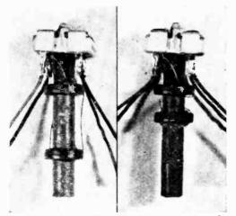
2. The original IF coil (left, can removed) can be modified by moving the windings closer.
