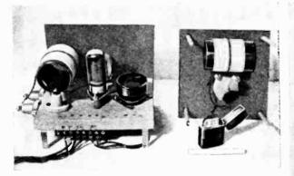
Legs for the transmitter are formed by twa metal angles in back, and the bottam of the panel in front. The two standoff insulators at the far left support the link-coupling coil, which is made of two turns of insulated wire around the center af the plate coil. Underneath the baseboard, mount the two R.F. chokes, the two by-pass condensers, and the 5,000-ohm cathade resistar, as shawn of the right.
