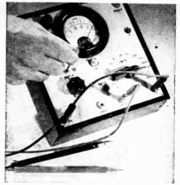
Adjusting the meter to read on the lowest ohm range. Scale divisions are graphed as below.
