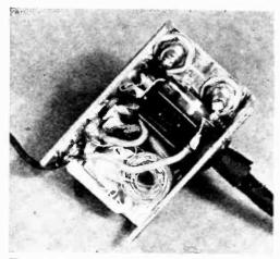
The turns of the antenna coil have been bunched together to take as little space as possible. An antenna lead and 4-way battery cable are brought out from under the chassis.
