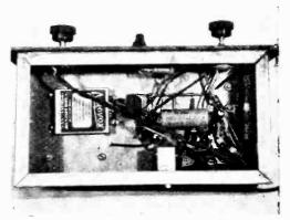
Subchassis wiring is comparatively simple. Test the various sections as you go along.
