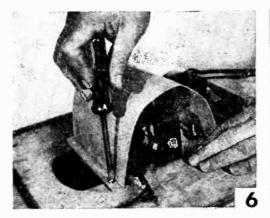
Sometimes the magnetic field set up by the motor persists even with all leads properly grounded. Should this happen, shield the motor with a thin sheet of ony magnetic metol ond ground the shield.
