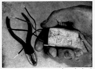
Many components can be purchased with tinned wire leads, all ready to solder into the set. Push about %" of insulation back from end.
