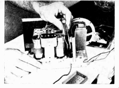
If the rectifier stack doesn't fit conveniently beneath the chassis, solder two extension leads to its terminals and install the disk over the empty tube socket.
