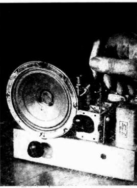
An alignment tool should be used for adjusting trimmers. Being nonmetallic, it can't short Bplus to ground. It also keeps hand capacitance from changing any of the circuit constants.
