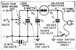
Wiring shown is for a metal chassis. To make the unit still safer, use a plastic panel, a DPDT switch, and connect all grounds together.
