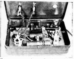
**Parts are mounted** on a flat chassis that is fastened inside the steel box by machine screws slipped through the rubber feet.
