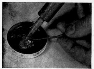
and dipping them into rosin flux paste. Put an end on a metal plate and run a thin coat of solder over it. Melt off any excess.
