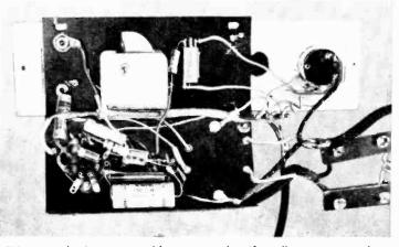
Wiring must be kept reasonably compact, but if small parts are used, no special crowding is necessary. Note the small 360-mmf. tuning condenser, and the miniature fixed crystol detector on its right.
