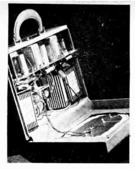
A piece of flat brass, cut to fit snugly ocross the upper part of the case, is used as a chossis. The lower portion of the cabinet is given over to the speaker and batteries. One 1.5-volt A and two 45volt B botteries supply the set with power. The loop antenna slips under the lid of the case.
