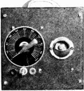
When correctly calibrated by the builder, this circuit tester will give accurate readings between 1.5 and 45 volts. The range can be extended by putting extra resistors in series with the potentiometer.
