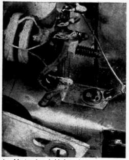
A soldering lug, held down by a screw that is used to fasten some other part to the chassis, provides an excellent ground connection.
