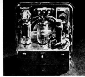
The plastic cover (removed in this view) is held to the chassis by the protructing screw.
