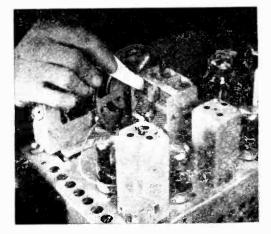
IN RECEIVERS where the oscillator and R.F. coils are not readily accessible for inserting a tuning wand, a strip of photographic film, old pyralin dial, celluloid, or similar material will serve handily. It should be thin enough to pass between rotor and stator plates without bending them.
