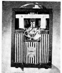
but does away with the C battery; the filaments of the tubes are wired for 1.4-volt operation. Place a small shield over the tube to reduce R.F. pickup from the tank coil.
