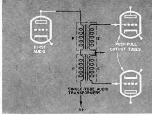
6. Two single-tube audio transformers make a neat replacement for a push-pull transformer.
