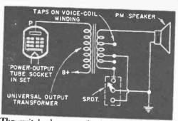
The switch shown at the left is wired across two taps of a universal output transformer. Select the best tap for each output tube.
