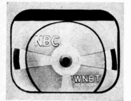
Vertical centering here just isn't centered. It would be the same if the picture went off screen at the top. This is also a rear control but is not made accessible on all types of receiver.
