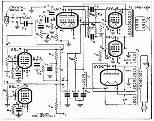
Two input circuits make it possible to leave both pickup and tuner permanently connected to the omplifier.
