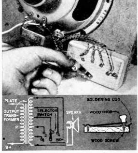
10. Selector switches are a cinca to make. A couple of screws and a flat metal arm do the trick. Use soldering lugs for the contacts.
