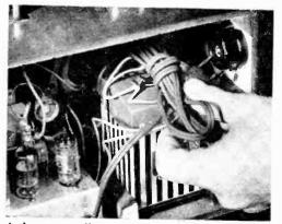
A dummy wall outlet is screwed to the side of the cabinet to provide an anchor for the AC-DC cord when the set is operated on batteries.
