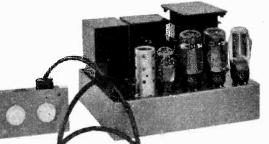
Leak TL-10, above, is king of the smaller amplifiers. A British import, on two chassis, it gives an utterly clean, clear 10 watts
