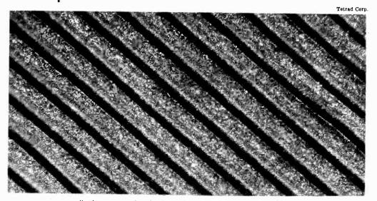
Here's a new record, as it appears through a microscope. Grooves seem straight because of the great enlargement necessary to obtain a readable picture of an item that's only .002 inch wide
