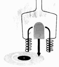
Here's a simple schematic of a magnetic pickup. The wires from the coils in which the current is " induced lead directly to necessary preamplifier
