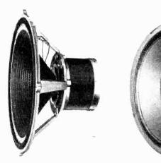
Wharfedale 12/CS/AL holds the paper-composition cone to the metal frame by means of a cloth suspension, lowering the speaker's fundamental resonance
