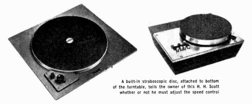
The Rek-O-Kut B-12H and B-16H feature hysteresis motors which govern the speed by the frequency of an alternating current rather than by line voltage
