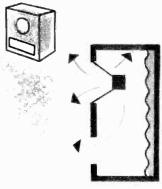
Bass-reflex box, most common kind of enclosure, brings rear waves around through port to reinforce the bass sounds from the front. Padding absorbs high-frequency rear waves
