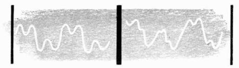
Here, graphically shown, is intermodulation distortion. At left is the correct pattern. At right is the uneven pattern produced when two frequencies, fed simultaneously into the system, distort each other
