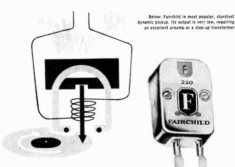
Above is schematic of dynamic pickup. As the stylus swings back and forth between the magnetic poles, the moving coll feeds out an alternating current
