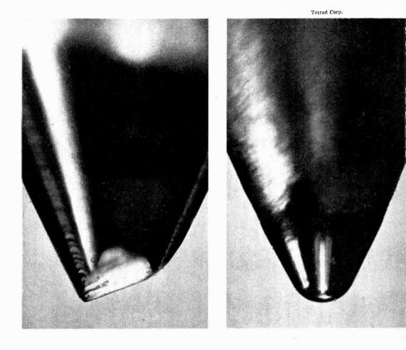
Sapphire stylus after 50 hours has lost its rounded tip and developed first tooth of its cutting edge. It will now damage records
