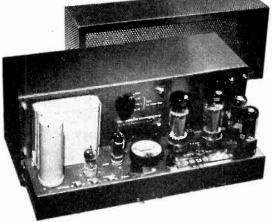
New Marantz has built-in meters for continuous testing of tube performance, produces 40 watts or 20, depending on circuit used. Rugged, conservative construction explains price of \$198
