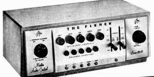
Push-button channel selector, volume controls for each input, up-down switches for turnover and roll-off are features of Fisher 80 panel design
