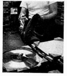
The resulting electroplate, peeled from the master, is a mirror image of the original, with ridges where the master bas grooves
