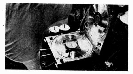
Forty seconds later a finished record emerges. The rough edge of surplus vinyllte will be sliced away later by an automatic knife while the next record is being pressed
