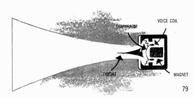
Operating according to fundamental acoustic principles, horn speaker uses a column of air to give audible volume to the vibrations of a voice coil is easily accessible to you, so that you are able to do your own balancing.
