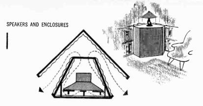
Klipsch design blocks the front of the speaker, brings front waves around to reinforce rear waves. Sound emerges from sides; corners of room form mouth of the horn
