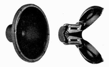
British-made Tannoy coaxial mounts the high-frequency horn behind the apex of the low-frequency cone, uses the curvature of the cone 80 to assure adequate dispersion of high-frequency sounds
