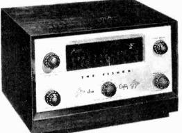
Left: Fisher 80-T tuner and preamp gives choice of inputs and equalization curves, AM or FM reception
