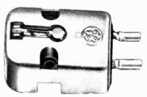
GE pickup comes in single-play (left) or triple-play models. A knob at top controls the swing of the bar to bring microgroove or standard stylus between the pole pieces
