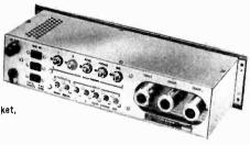
Simple sockets for simple plugs make electrical connections easy. Cable from pickup goes into the MAG socket, and a two-plug cable runs from output socket to amp
