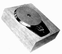
Components Corporation isolates motor from the record, conveys the necessary power by means of belt around the turntable
