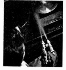
Master record is coated with a silver solution to make it an electrical conductor and prepare It for the electropiating vat
