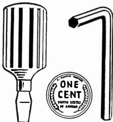
Fig. 8. You may operate the captive studs that hold the replaceable units together, by the familiar Allen Wrench, a screw driver, penny or dime.
