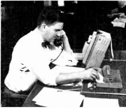
This 2" facsimile desk scanner of Alden Products Co. is a great boon to central and branch bank operations.
