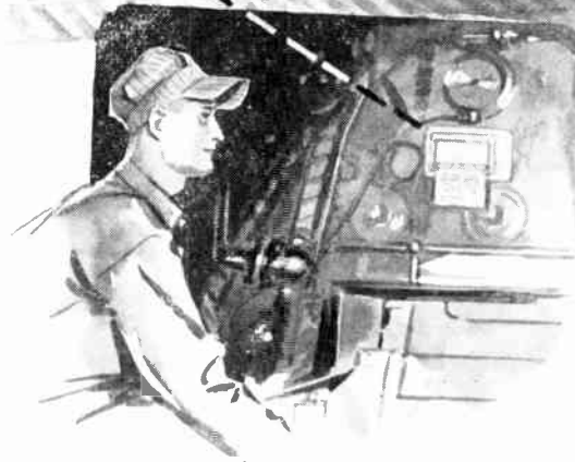
The Alden Dispatch Recorder in a locomotive cab can be read by the engineer while busy with locomotive operation. The transmitting scanner may be at a station, signal tower, or in the rear of the train.
