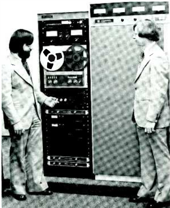
Harris has exhibited its CPM AM stereo system at the 1977 and 1978 NAB and NRBA Conventions. Dave Hershberger (1) and Cliff Leitch, design engineers for CPM, are shown in front of a Harris MW-1A, one-kilowatt AM transmitter, operating in stereo.
