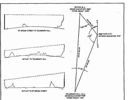
Fig. 19—Triangular relay system on which much experimental data were obtained. The terminal is at the southerly tip of Manhattan Island in New York City. Two repeaters are located at Nutley and Telegraph Hill, both in New Jersey. Overland and overwater links are thus included.
