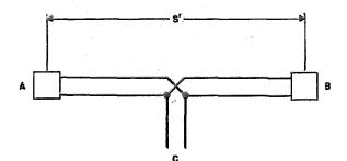
Fig. 1—A two-element array or directional pair equally applicable, from the standpoint of field pattern, to the transmitting or receiving cases.
