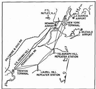
Fig. 4—Map showing locations of the four stations comprising the New York City-to-Trenton circuit.
