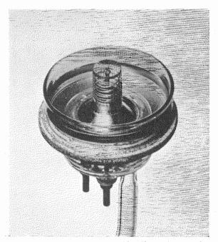
Fig. 5—Grid and filament assembly. The grid connecting ring and cone support may be clearly seen.
