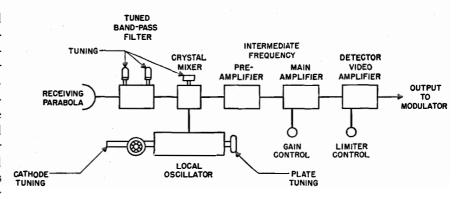
Fig. 2-The receiver consists of the components indicated in this block diagram.
