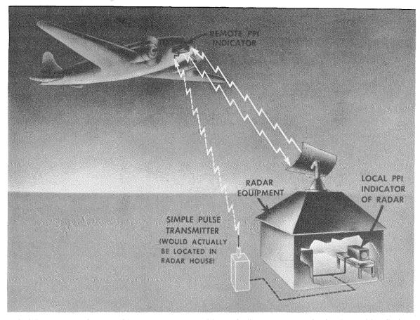
Principle of remote radar as used for the Navascope, or airborne duplicate of the ground radar plan-position display.
