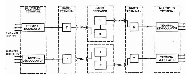
Fig. 1—Disposition of equipment in a radio relay system. R = receiver and T = transmitter. Only one repeater is shown; additional repeaters may be included.
