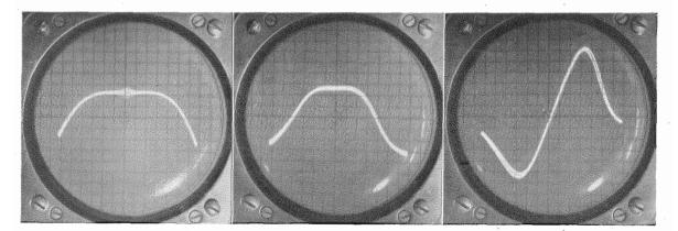
Fig. 15—Three oscillograms obtained from the auxiliary receiver of the transmitting equipment. The first two curves are the response-frequency characteristics of the intermediate-frequency amplifiers. The bandwidths are 2 megacycles. The discriminator response-frequency characteristic is displayed in the oscillogram at the right.
