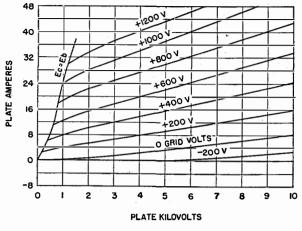
Fig. 7—Average plate characteristics of the 7C27.
