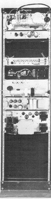
Figs. 10 and 11—Front and rear views of radio repeater rack in which both the receiver and transmitter assemblies are mounted.
