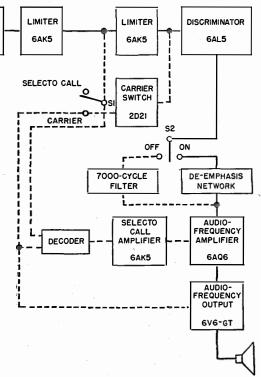
process, the 7000-cycle subcarrier is discarded and, if the lower-frequency modulation is of the proper frequency, the decoder operates. The decoder is essentially a single-pole single-throw switch, which is normally in the open position. When the decoder is actuated, the switch is closed and the audio-frequency system becomes operative.
