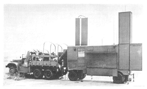
Wartime model of a mobile ground-controlled-approach (GCA) installation. Power and air-conditioning equipment is in truck at left; radar and communication antennas are seen on the roof and side of the trailer unit. The trailer contains all equipment and indicators required to enable the operators to "talk down" an airplane.
