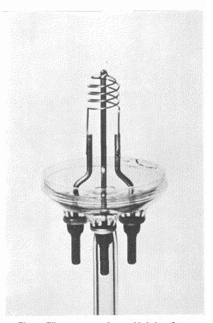
Fig. 4-Filament mounted on molded glass flare.
