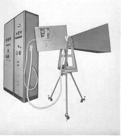
Fig. 4—Transmitting equipment. The microwave transmitting tube and radiating horn are mounted on the tripod for convenience in aiming.
