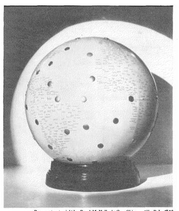
Base map copyright by Rand McNally  $\cong$  Co., Chicago, Ill., R.L. 4728. Globe view showing possible locations of ground transmitters of 1500-mile range, for providing radio navigational service at all points in the North and South Atlantic oceans.
