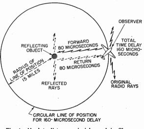
Fig. 4—Absolute-distance principle used in Shoran system.
