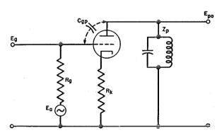
Fig. 4-Variable-transconductance phase-shift modulator.
