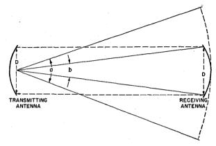
Fig. 1—Free-space attenuation is a function of the beam characteristics of the antennas. The angle in which the radiation is concentrated when using dipole radiators and parabolic reflectors is  $a = 1.7 (\lambda/D)$ . The angle in which the receiving antenna is viewed from the transmitting point is b = D/L, where L is the distance between wansmitting and receiving antennas.
