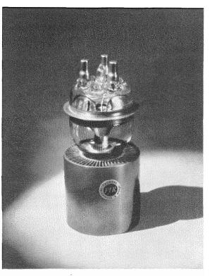
Fig. 4—7C27 air-cooled triode capable of giving 5 hilowatts of power at 110 megacycles.
