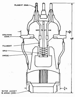
Fig. 2—Cross-sectional view of 6C22.
