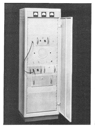
Fig. 10-Remotely controlled land-station 250-watt transmitter and receiver, "front door open.
