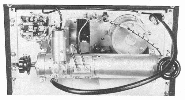
Fig. 7—Rear view of transmitter. The tuned coaxial oscillating circuit is at the bottom. The screw-feed adjustment at the left is for plate-circuit tuning. The cathode tuning control is at the right.
