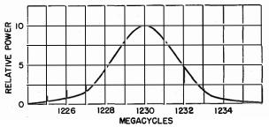
Fig. 8—Frequency variation of transmitting and receiving oscillators during 7 hours in which the temperature was changed from 0 to -38 to +60 degrees centigrade.
