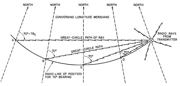
Fig. 3—Direction-finding complications at long distances.  $TB_r = TB_t + 180$  degrees + meridian convergence correction.
