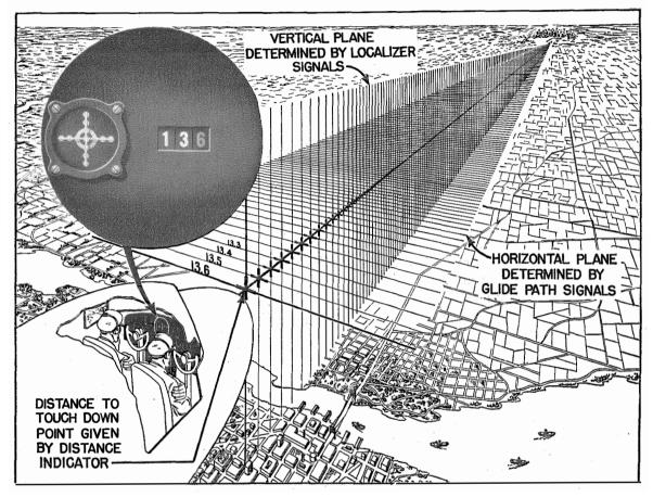
Fig. 10-Instrument landing system principle used in Navaglide.
