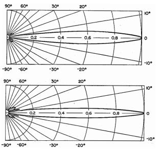
Fig. 15—Horizontal and vertical directivities of a 1400megacycle (21.4-centimeter) dipole in<sup> $\tau$ </sup>a 10-foot parabolic reflector. Relative voltage output is plotted against angle of radiation. At the top, the directivity is measured with the dipole horizontal, while below it is vertical. Half power (3 decibels down) is equivalent to 0.7 relative voltage.
