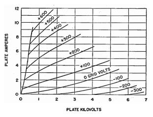
Fig. 3—Average plate characteristics of the 7C26.
