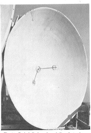
Fig. 14—Typical dipole and parabolic reflector for use in the 1000- to 3000-megacycle region. The enclosure around the dipole protects it from rain, snow, and sleet.
