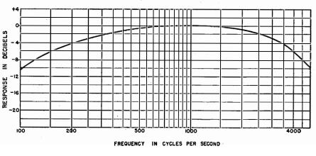
Fig. 2—Response-frequency characteristic of the mobile equipment. Reference level is the response at 1000 cycles.
