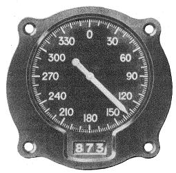
Simple meter type of presentation for an  $R\theta$  radio navigational system. Distance in miles and tenths is shown by the number-wheel type of indicator; bearing or azimuth is shown in degrees by the pointer. As distance and bearing are indicated simultaneously from the same radio landmark, complete information for a position fix is constantly presented in direct terms.
