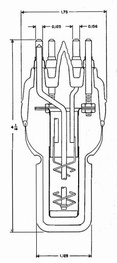
Fig. 2—Plan drawing of the 7C26. There are six base pins, three of which are connected by short leads to the grid structure. The other three are for the thoriatedtungsten filament and its center tap. The radiator is not shown.
