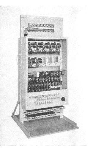
subgroups. The number of paths in the groups being observed need not be in multiples of 10. If some of the arc contacts of the selector switches are not connected to circuit paths, tests in these positions will of course never cause an operation of the message register, and the traffic recorded will be that on the paths connected through terminals of the recorder to the selector arcs.
