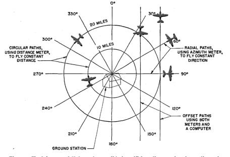
Fig. 11—Useful types of flight paths possible in an  $R\theta$  or distance-bearing radio navigational system. Tracks may be accurately followed by reference to a distance-azimuth meter like that shown in a previous illustration.
