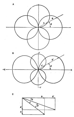
Fig. 10—A perfect set of figure-of-eight patterns are shown in A. In B the patterns are not symmetrical. The vectors in C illustrate the correction  $\beta$  which must be applied to the indicated bearing to obtain the correct bearing.
