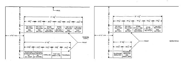
Fig. 9-Possible floor plan of the terminals and of the repeater.
