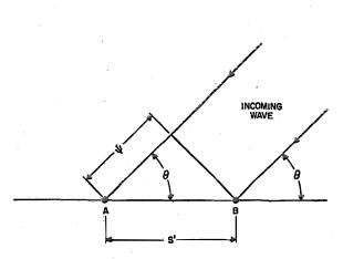
Fig. 2—Factors involved in calculating the receiving pattern of the two-element array (Fig. 1).  $\theta = \text{angle of reception to plane of array. S' = spacing angle = 360 S/<math>\lambda$ , where S = actual spacing.  $\psi = S' \cos \theta$ .
