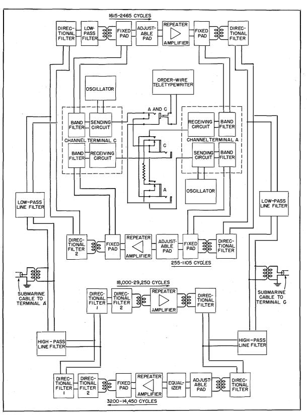
Fig. 3—Schematic arrangement of Repeater B equipment.
