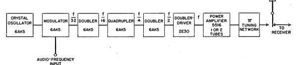
frequency multipliers which operate as saturated class-C amplifiers. The output of the power amplifier stage, also operating class C, is coupled to the antenna through a tuned  $\pi$  network. The transmitter may be operated at any frequency between 30 and 44 megacycles by inserting a crystal of the proper frequency and adjusting the tuned circuits.
