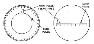
Fig. 5—Principles of two common ways of displaying on a cathode-ray tube the time interval between pulses. Graduations may indicate time in microseconds or the corresponding distance in miles.
