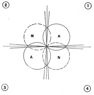
Fig. 8—Principle of the A-N radio range system showing the two figure-of-eight patterns alternately radiated and the four equisignal sectors or beams. fixes by means of intersecting beams from other stations are only occasionally possible. The four beams sound alike, so if the pilot is completely lost, considerable ingenuity and time are required to judge which of the four beams he is on—if at all possible.
