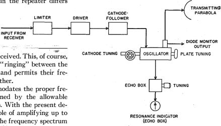
Fig. 5—Block diagram of transmitter. The modulation is applied to the oscillator through the cathode-follower. The tunable cavity resonator (echo box) and resonance indicator are used to monitor the output radio frequency.
