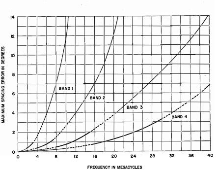
Fig. 9—Maximum spacing error in arrays covering 1.5 to 30 megacycles in four bands. The heavy solid line indicates the nominal range for each band, the dotted line indicates the extended range, and the light solid line shows errors which occur outside the range of each band.
