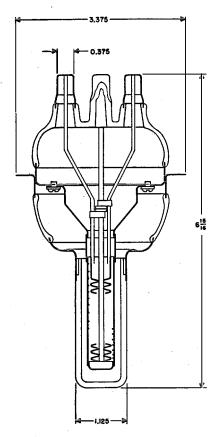
Fig. 5—Plan drawing of the 7C27. The radiator is not shown.
