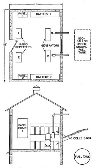
Fig. 13—Power plant for unattended repeater station.
