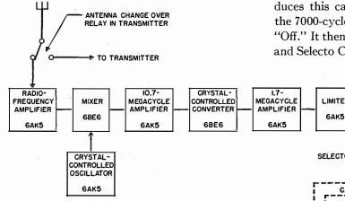
Fig. 6—Schematic arrangement of the receiver. The units connected by solid lines comprise a conventional double-conversion superheterodyne circuit. The broken lines connect the Selecto Call and squelch circuits.
