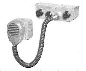
Fig. 1—The mobile receiver and transmitter are mounted in the cabinet and may be placed in any convenient space in the automobile. The microphone and control box are usually mounted on the instrument board.
