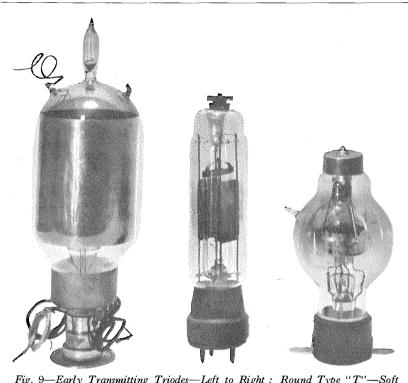
Fig. 9—Early Transmitting Triodes—Left to Right : Round Type "T"—Soft Vacuum, 1914 ; Telefunken Type R.S.5, 1919 ; Marconi-Osram Type M.T.3.
