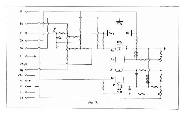
decoupling condensers for the cathode and for No. 2 anode are of the same type and are used for the same reason as those already referred to in connection with the mains unit. The rest of the circuit is self-explanatory.
