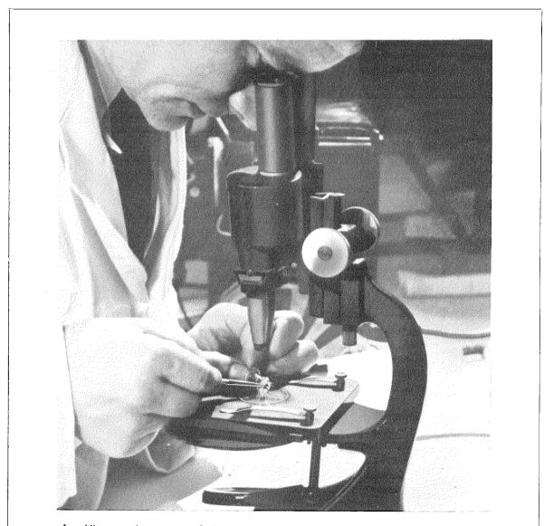
Assembling a centimetre-wave tube having an anode with a radius of eight-thousandths of an inch. Because of its small size, this type of tube is assembled under a binocular magnifier. (Les Laboratoires, L.M.T., Paris.)
