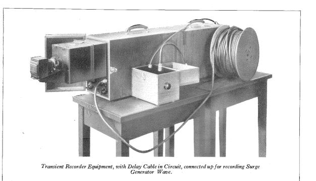
of focus with writing speed, and high plateconductivity with large values of positive deflecting voltage. With the advent of the high-vacuum tube it became possible to produce a much more stable and reliable apparatus, capable of recording at considerably higher writing speeds.
