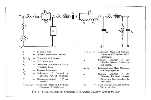
An advantage of the new receiver, due to its damped characteristic, is that the effect on the ear of surges or any abrupt interfering noises in the listener's circuit is much reduced. The energy of a surge tends to set the diaphragm in motion and, when the latter is freely resonant as in the old receiver, the motion persists for several cycles; in a well damped diaphragm system, however, the surge energy is dissipated too rapidly to be fully appreciated by the ear.
