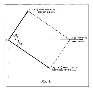
and end of a signal, as indicated diagrammatically by the rotating vectors in Fig. 5. Considering the intensities of the signals, the equation becomes more involved; separating the real amplitudes a and the phases  $\varphi$ :
