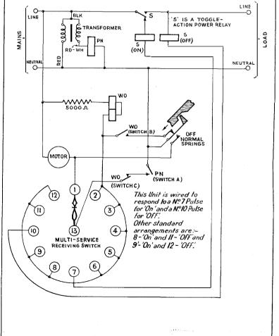
Fig. 9-Schematic Circuit of Multi-service Control Receiving Unit.
