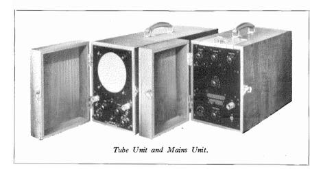
a terminal connected to the central electrode for the tripping impulse. On the front of the tube unit are the modulating control, focus control, biasing controls for X and Y plates, and a push button which, when operated, applies a pulse to the central electrode to trip the spark-gap artificially.
