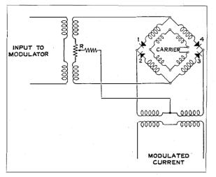
Fig. 3—Modulator Schematic.
