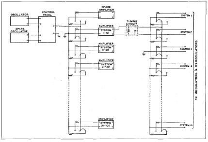
Fig. 4-Block Schematic of Carrier Current Supply.
