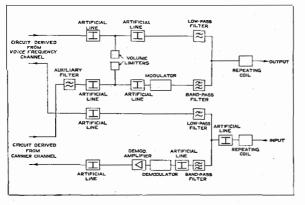
Fig. 1-Block Schematic of Single Channel Carrier System.
