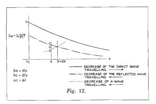
The approximation indicated by the sign  $\approx$  consists in *neglecting the attenuation on a length* r: the term  $\beta r$  is presumed to be negligible, account being taken only of  $j \alpha r$ ; the cable irregularities will always be sufficiently short to justify this approximation, even if the length r or l attains some hundreds of metres.
