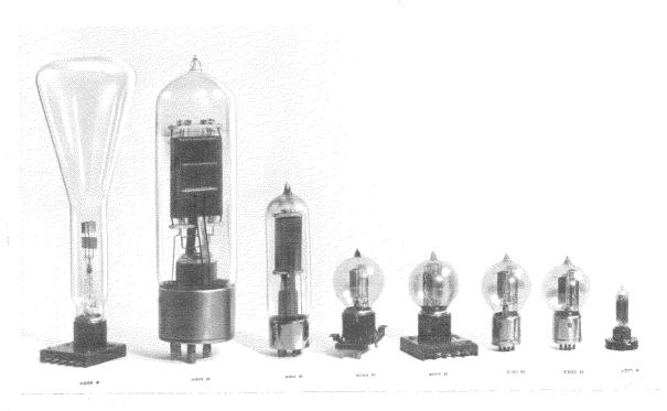
Fig. 7—A Range of Oxide-coated Alloy Filament Valves made by Standard Telephones and Cables, Limited.
