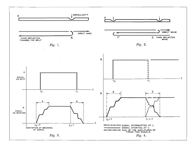
Fig. 4. The curves of growth and decay must therefore be exactly complementary.
