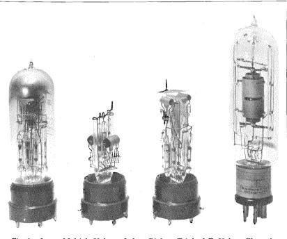
Fig. 8—Loewe Multiple Valves—Left to Right : Triple A.F. Valve—Electrodes of Double R.F. and Triple A.F. Types ; Siemens-Halske Schottky Tetrode, Type O.R.
