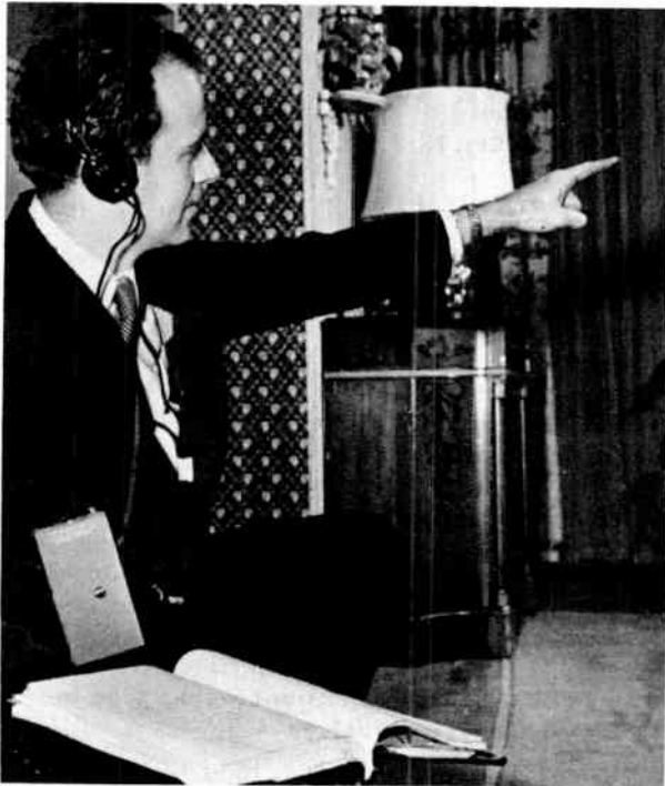
Fig. 34 Communication to the studio floor manager, as well as other studio personnel who must be free to move to any part of the studio, is accomplished by means of a low-frequency induction-field transmission channel. One of the compact receiver units is shown in this photograph.
