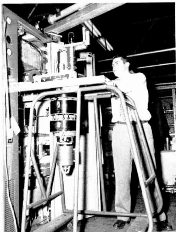
Fig. 6 Klystron mounted on dolly, ready for installation in transmitter.
