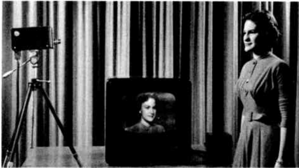
Fig. 7 Camera adapter in use with standard television receiver.
