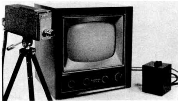
Fig. 1 Camera adapter with receiver and control box.
