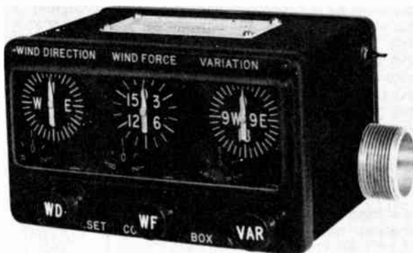
Fig. 3 Preset control box.
