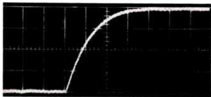
Response to a current step of 10^{-12} amp. Input capacity is 35\mu\mu\text{f} . One major horizontal division equals 200 milliseconds.
