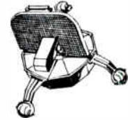
Solar Observatory —350 lb. Large flywheel and extended arms rotate to stabilize. Under construction.
