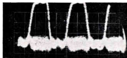
Fig. 10—Photograph showing both biasing wave form (large square wave) and PLO output modulated at 140-Mc rate.
