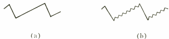
Fig. 31—(a) Horizontal scanning wave applied to vertical wires. (b) Vertical scanning wave applied to horizontal wires.
