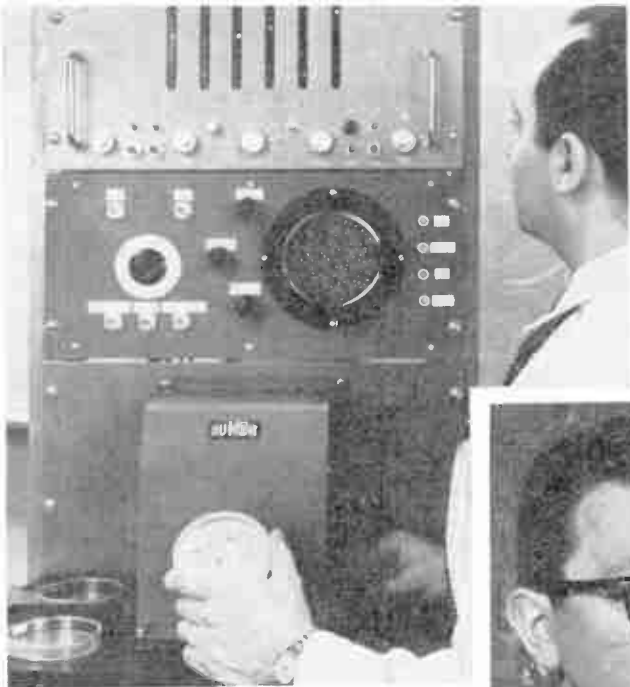
Above —The New DuMont Inconumerator can, in one second, count up to one million objects of varying shapes and sizes. Here, the device is operated by DuMont engineer, H. P. Mansberg who, with Carl Berkley, supervised Inconumerator's design and construction.
