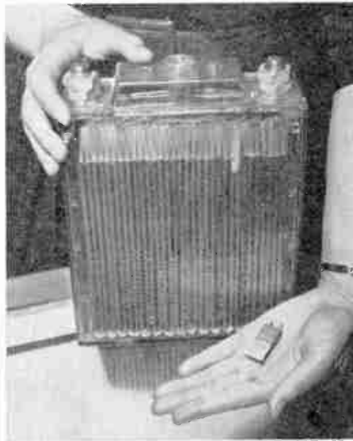
Above —Tiny storage battery weighing one-sixth of an ounce is, according to Yardney Electric Corporation, the world's smallest. Here it is compared with one of the largest single-cell units made.
