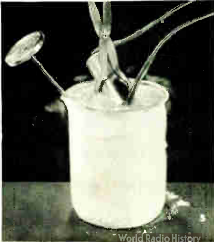
5. At -55 degrees centigrade, the subminiature G-E metal-clad capacitor with Permafil dielectric shows less than 7 percent loss in capacitance.
