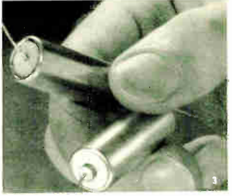
3. Undamaged by dropping, the two capacitors are shown here—note that there are no cracks in the G-E silicone-sealed unit.
