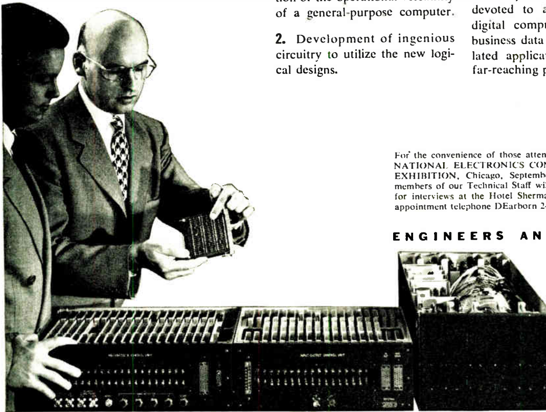
One of the subminiature switching circuits from the Hughes airborne electronic digital computer is examined by Dr. Eugene M. Grabbe (right), Associate Head, Computer Systems Department, Advanced Electronics Laboratory, and Phil A. Adamson of the Technical Staff.
