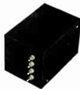
This ultra low frequency filter has a band pass range of one cycle to 10 cycles... 50,000 ohms... 700 cubic inches.
