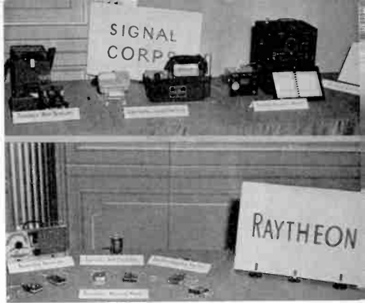
Top —Conventional equipment compared with smaller transistorized versions. From left to right: A wire repeater, Geiger counter, and frequency meter. Bottom —Transistor equipment including a radio receiver, test oscillator, "phone-plug" amplifier, and several hearing aids.
