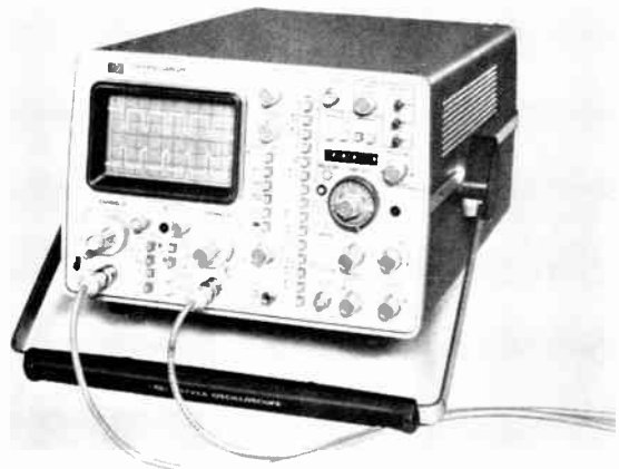
[1] The LED display on Hewlett-Packard's model 1722A microprocessor-based oscilloscope indicates the period of the waveform under observation. The use of a microprocessor also allows highly accurate display of analog-trace voltage magnitude, the time interval between traces, and signal frequency, as well as a number of other parameters.
