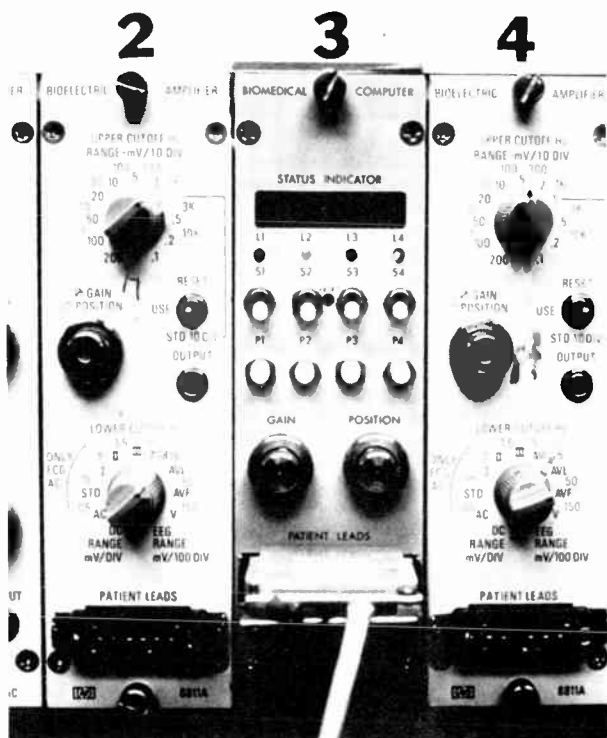
[3] The entire general-purpose, biomedical computer system developed at the VA Hospital in San Diego, Calif., fits into the plug-in module of a strip-chart recorder.
