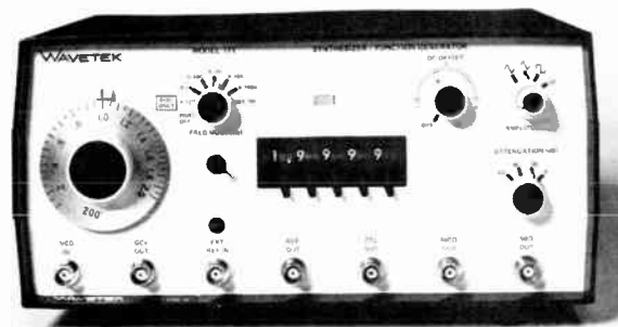
[5] Wavetek's model 171 synthesizer/function generator is a low-cost solution to improving the performance of traditional function generators. It is basically a synthesizer with excellent function-generator performance levels.
