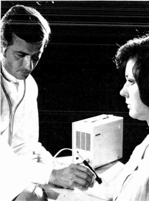
Noninvasive blood-flow velocity indicator by Siemens operates at ultrasonic frequencies using the Doppler effect. With this instrument, stenotic disorders or functional incompetence of the venous valves can be diagnosed rapidly.
