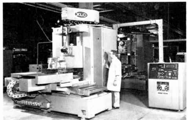
Ex-Cell-O 408 Work Center controlled by General Electric's computer numerical control—Mark Century 1050.
