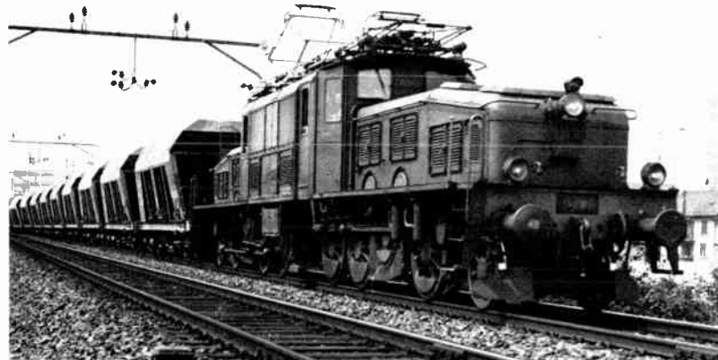
[3] One of the famous Class Ce 6/8 11 "Crocodile" freight locomotives, originally built between 1920 and 1922 for service on the Gotthardbahn. Weighing 131 tonnes, with a rating of 1840 kW, they are still going strong in 1974, as may be seen by the modern high-rise structure at the right center of the photo. Thirteen more of these machines, designated Class Ce 6/8 111 , were built in 1926–27.
