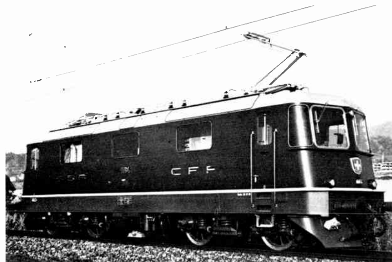
[4] An Re 4/4 11 (two-bogie, four-axle) high-speed passenger locomotive of the SBB. A modified version of this 4600-kW machine is a thyristor-controlled locomotive used on BLS service. The Re 4/4's have been built since 1964.
