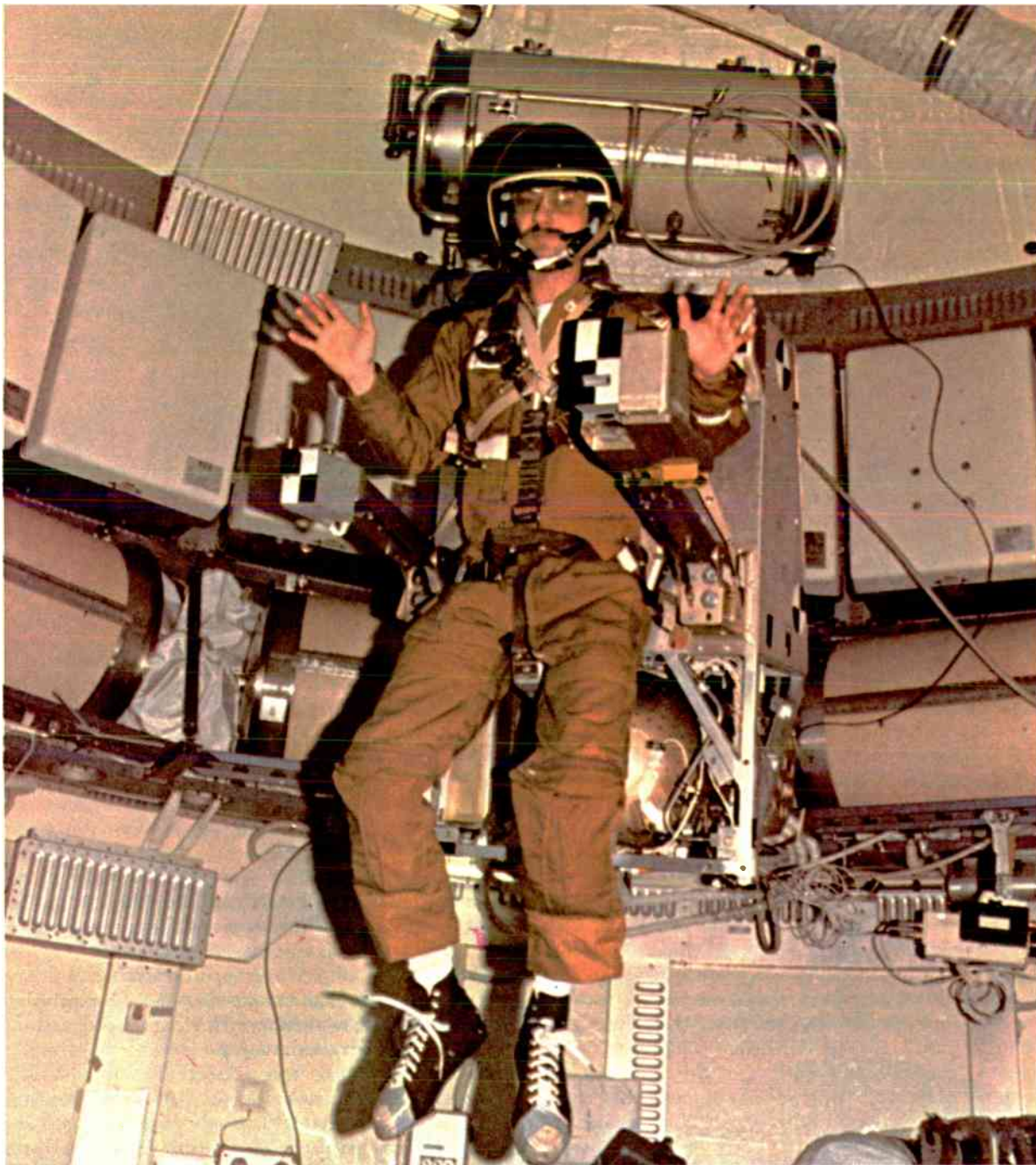
Astronaut Garriott flies the experimental maneuvering equipment in the forward dome of the Skylab orbital workshop, thus demonstrating man's maneuverability in zero gravity.
