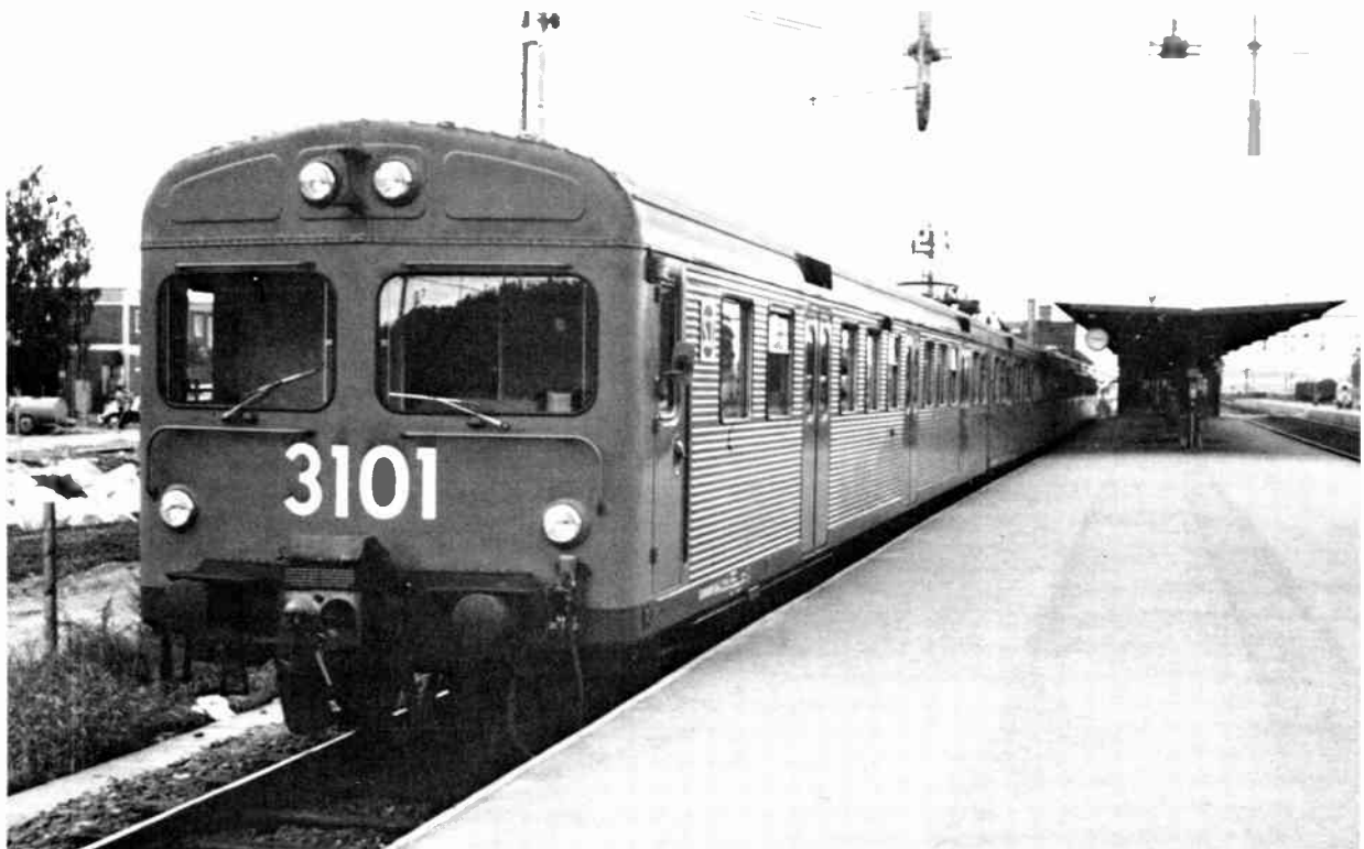
[6] Train of two-coach Class X1 sets is shown in the station at Marsta, a suburb of Stockholm.
