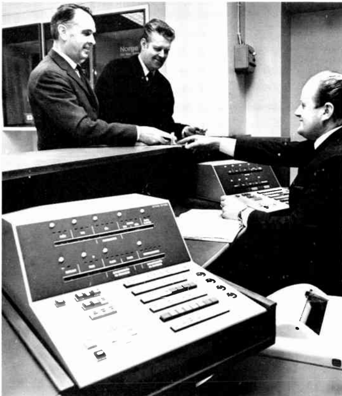
[9] Computer terminal at Stockholm's Central Station ticket booking office is part of extensive automated ticket issuance and accommodation network employed by the SJ. When a passenger requests a specific day, train, and compartment, the booking clerk keyboards the order. In 15 seconds' time, the ticket, or seat reservation, is printed out.
