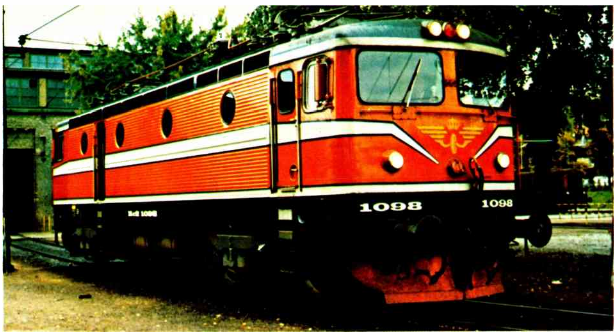
[2] "Showcase" unit of the SJ—the ASEA-built class Rc 2 thyristor-controlled locomotive is used for mainline passenger express service, primarily in Sweden. Similar (diode) versions of this locomotive have been exported to Yugoslavia, Romania, and Norway for mixed traffic (freight and passenger) service. Thyristor locomotives, similar to the Rc 2, were sold to Austria.
