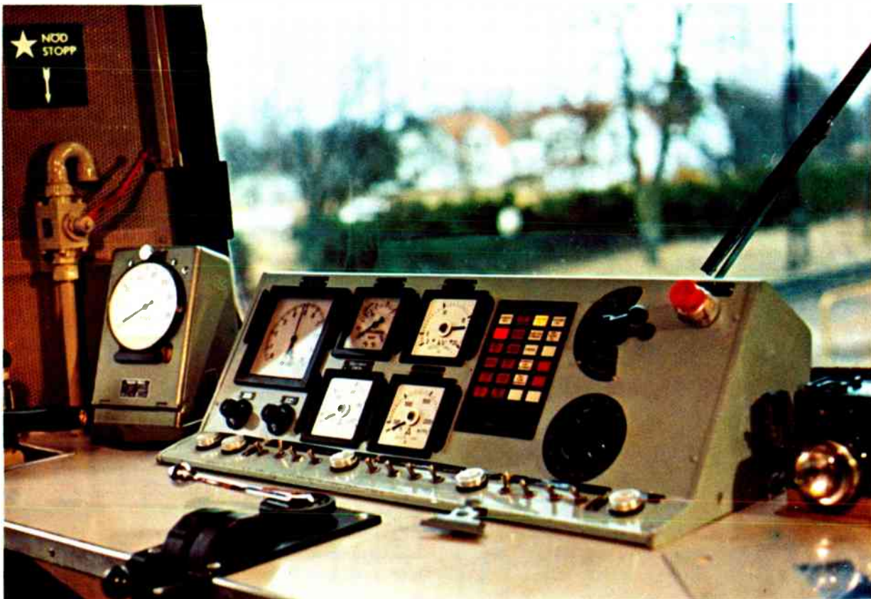
General view of driver's cab of Rc 2 locomotive, showing the instrument console and the tractive effort control lever, located on the desk below the center of the instrument panel.
