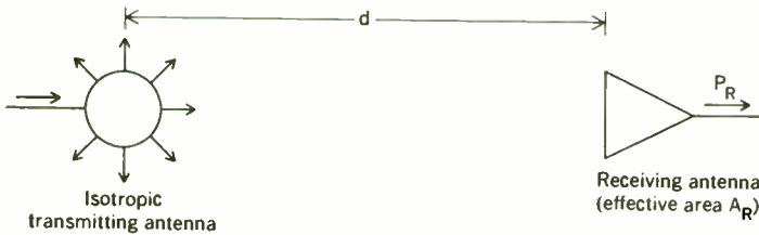
FIGURE 15. Relation between the gain and the effective area of an antenna.
