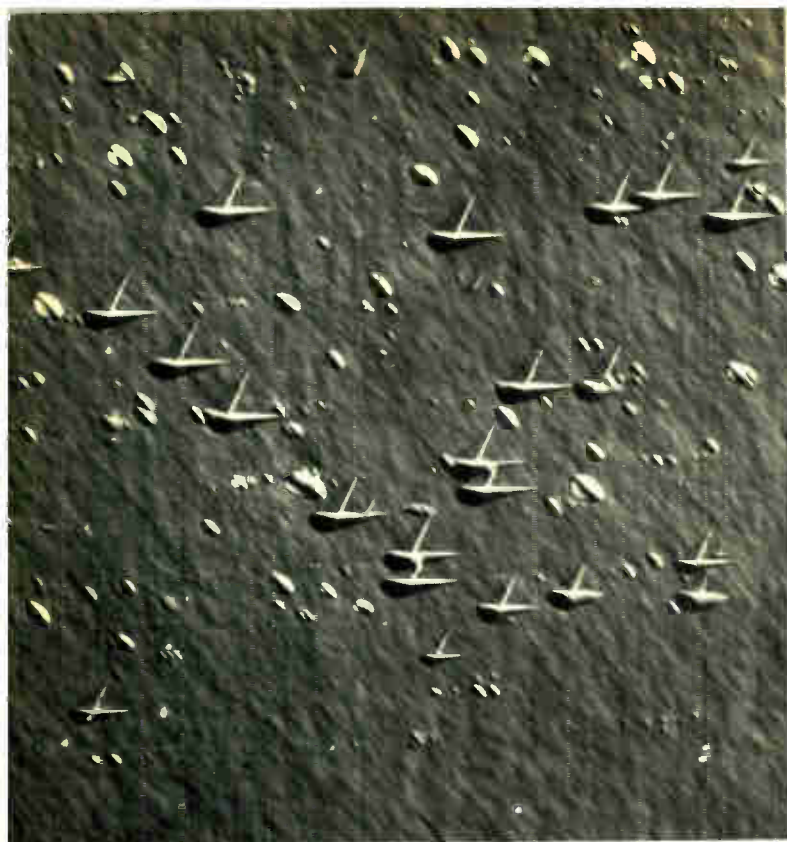
Only with Epi-Nomarski Interference Contrast do faults such as these in unetched silicon crystals stand out. (200x)
