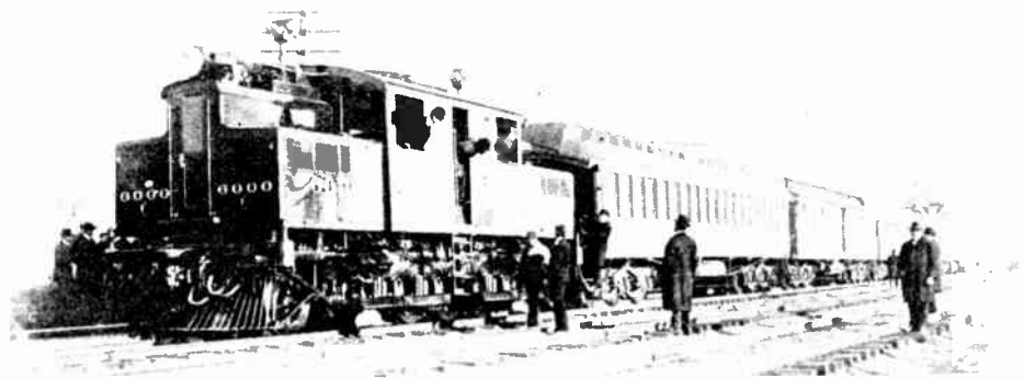
FIGURE 10. The GE-built 86-tonne electric locomotive on its official test run, November 12, 1904. This was the prototype of a series of steeple-cab engines specially built for the New York Central Railroad. A few of these early locomotives are still in yard service.
