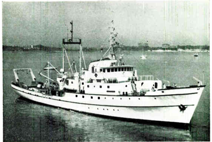
Fig. 2. The U.S. Bureau of Fisheries' specially designed research vessel, "Albatross IV," is the first stern-ramp trawler built in the United States. The ship is completely equipped with biological and chemical laboratories for the acquisition of marine scientific data.
