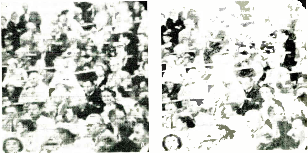
Fig. 3. Pictures of a crowd received through simulated PCM systems. A— 128 \times 128 samples; 64 brightness levels. B— 256 \times 256 samples; 16 brightness levels.
