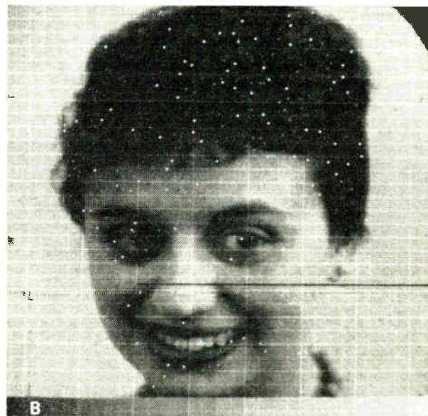
Fig. 5. Picture received through binary symmetric channel with p = 0.003 , using (A) natural code and (B) Gray code.
