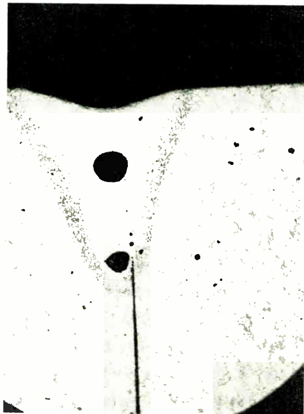
Fig. 10. Laser weld of two pieces of stainless steel.
