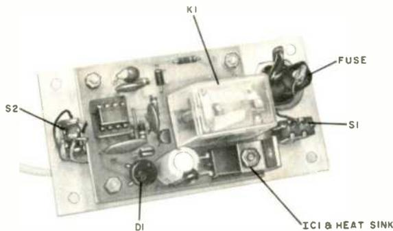
Fig. 4. Photo of prototype printed circuit board removed from enclosure.
