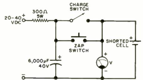
Fig. 2. Shorted cell is cleared by energy stored in capacitor.
