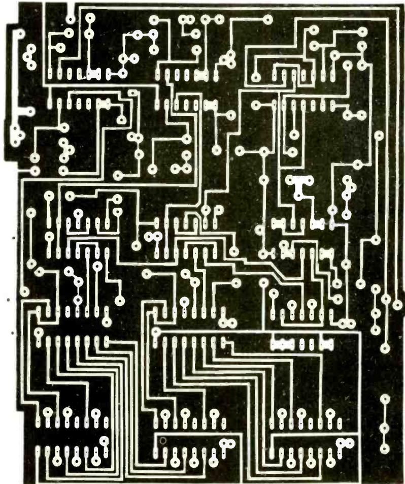
Fig. 2. Pcb board etching and drilling and component (top) guides.
