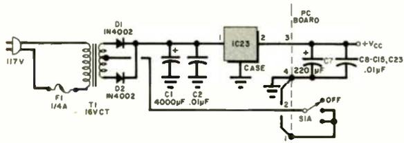
Fig. 6. Power supply circuit has a voltage regulator IC.
