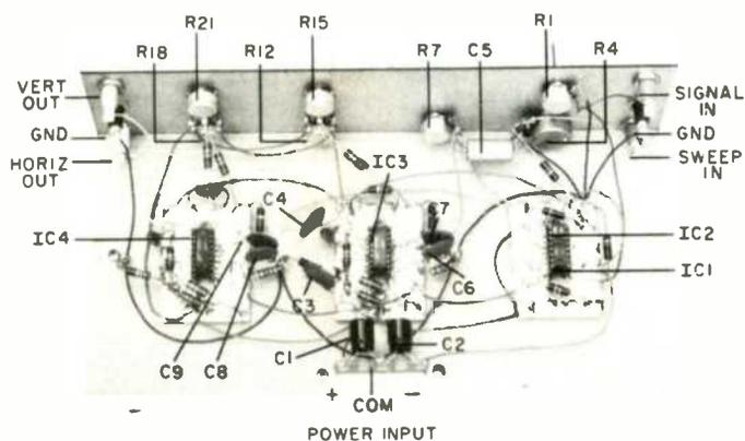
Fig. 4. Photo at top shows front panel of prototype. Below is prototype breadboard. Pcb board can be used.
