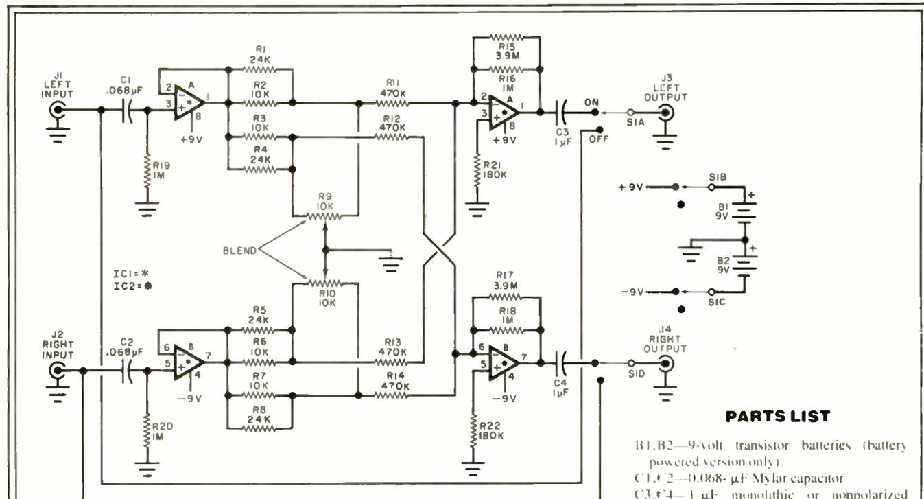
Fig. 1. Schematic diagram of the stereo blend.
