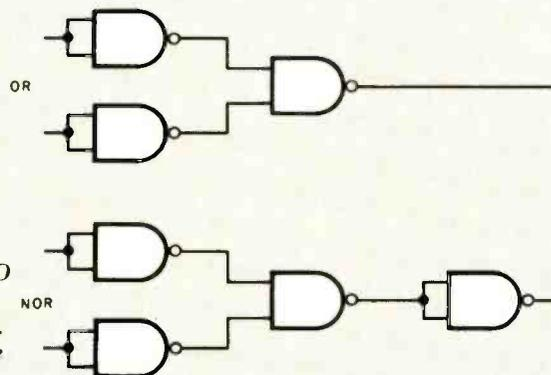
**Complex Logic Systems.** Simple and compound gates can be tied together to implement a countless variety of logic functions. Some of the resulting logic systems contain only a handful of gates; others may use dozens or even hundreds of gates. All of these complex logic systems can be divided into two broad categories: combinational and sequential.
