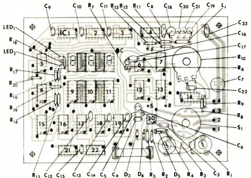
Fig. 8. Component placement guide. Numbered circles are feedthroughs.
