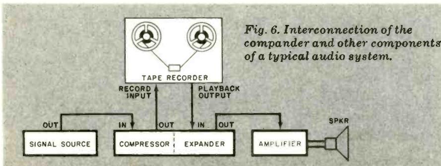
Fig. 6. Interconnection of the componder and other components of a typical audio system.
