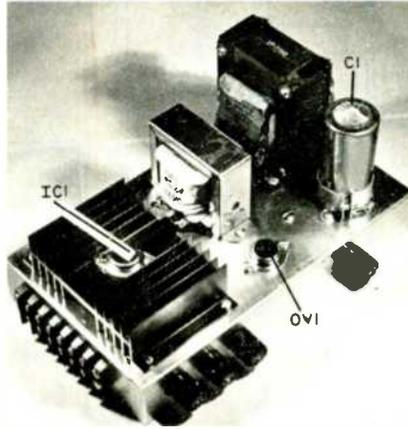
for the voltage regulator so that it will run cool at its full rated current.
