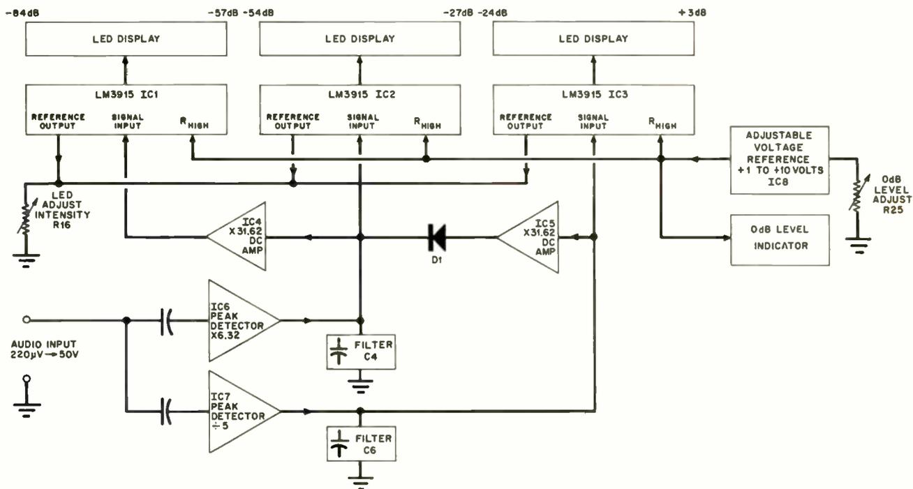
Fig. 2. Block diagram of one channel of the Wide-Range Audio Meter.
