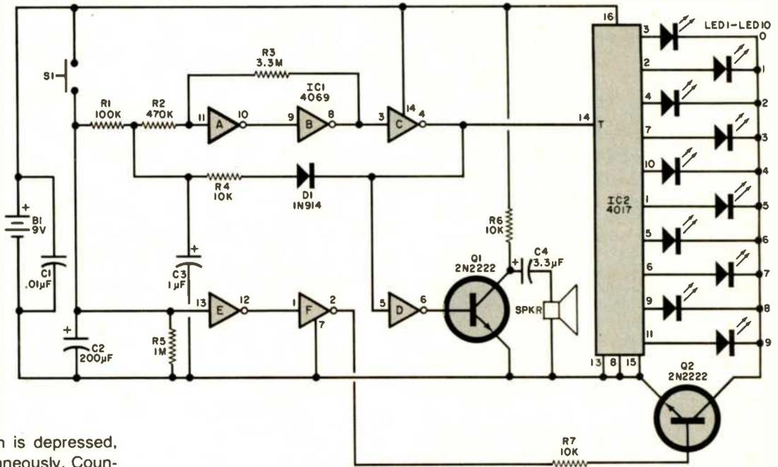
When the pushbutton is depressed, two things occur simultaneously. Counter IC2 is reset to zero by the signal on pin 2, thus placing all of the IC2 outputs at their low states (0 volt). Thus, none of the LED's can glow. The second action is an enable level signal (+9 volts) at pin 13 of IC1. This action allows the oscillator (the middle two gates) to start, thus producing an input signal to the counter IC through the last gate of IC1.
