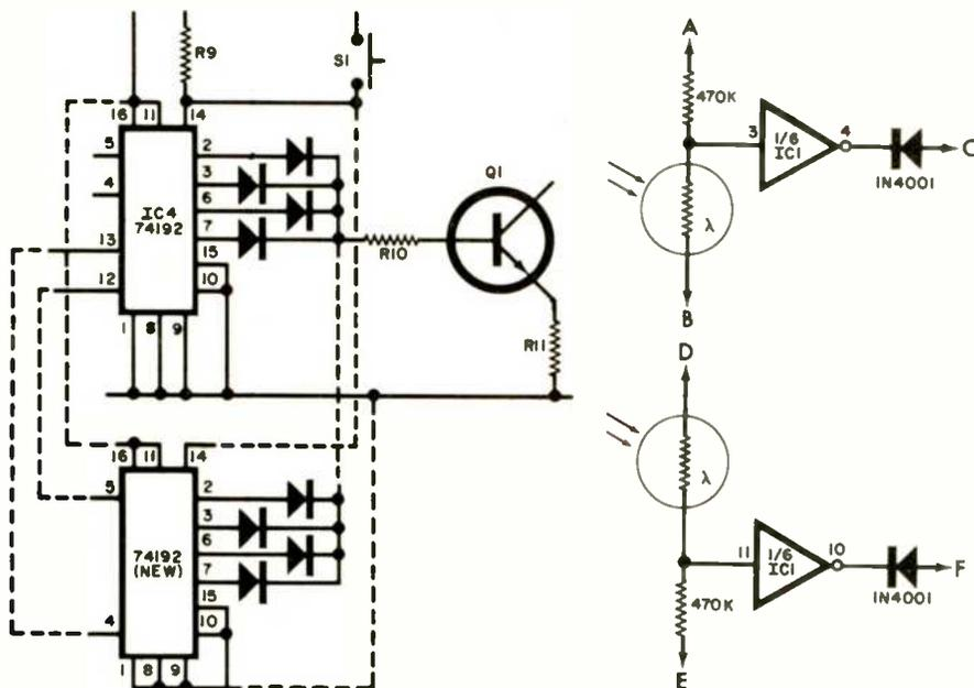
Fig. 2. Count can be increased by adding another up/down counter.
