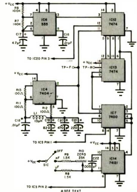
Fig. 3. Oscillator, sync., and reset circuits.
