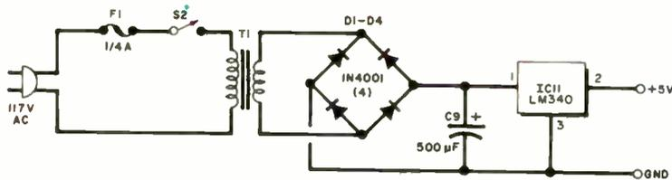
Fig. 4. Ac supply for low-power "Charge!"
