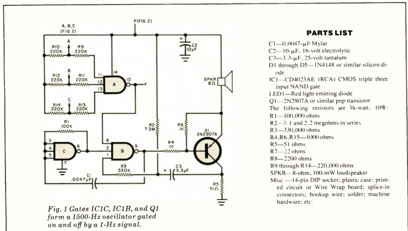
*Fig. 1 Gates IC1C, IC1B, and Q1 form a 1500-Hz oscillator gated on and off by a 1-Hz signal.*
