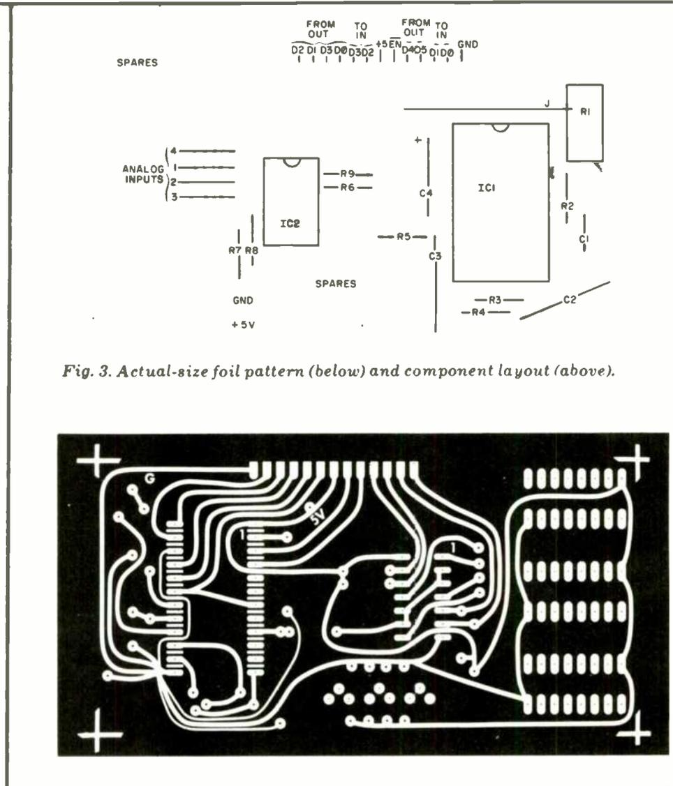
Fig. 3. Actual-size foil pattern (below) and component layout (above).
