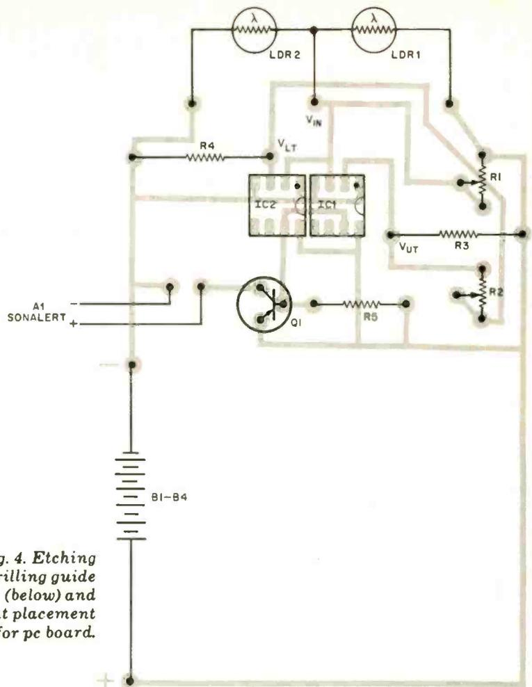
Fig. 4. Etching and drilling guide (below) and component placement for pc board.
