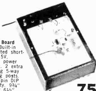
Proto Board 203. Built-in regulated short-proof 5V, 1-AMP power supply. 2 extra floating 5-way binding posts. 24-14 pin DIP capacity. 9 $\frac{3}{4}$ " long x 6 $\frac{1}{2}$ " wide x 2 $\frac{3}{4}$ " high. All metal construction.
