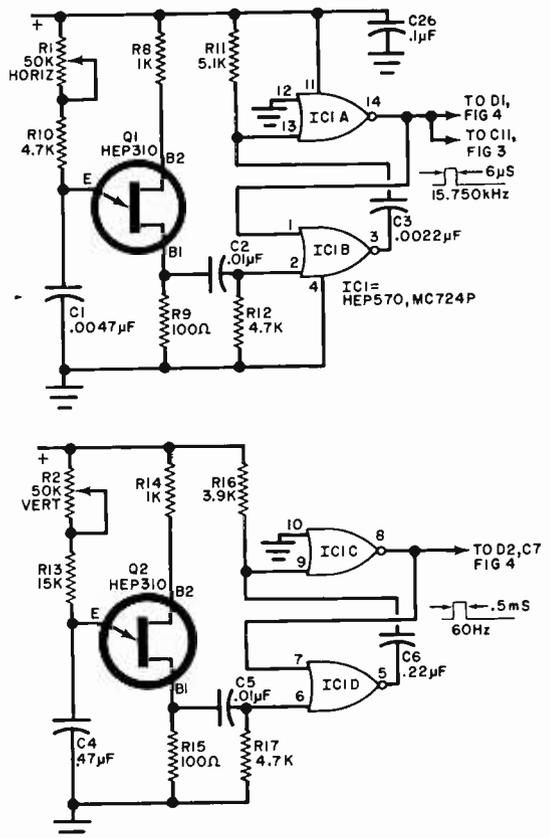
Fig 2. Horizontal and vertical oscillators feed one-shot multivibrators.
