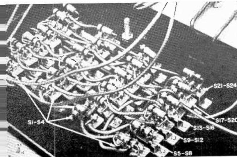
The bulk of the work is in cutting the holes to mount the 24 switches in the selector circuit. Be careful when drilling plastic as it shatters very easily. If there is any doubt, use a metal cover for the plastic container.
