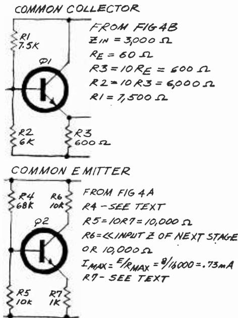
The input impedance of the emitter amplifier is  $R_{IN}$  (3600) in parallel with 25,000 or 3000 ohms, which is what is desired. If the values were found to yield an overall input impedance which was not 3000 ohms, the components would have to be adjusted appropriately.
