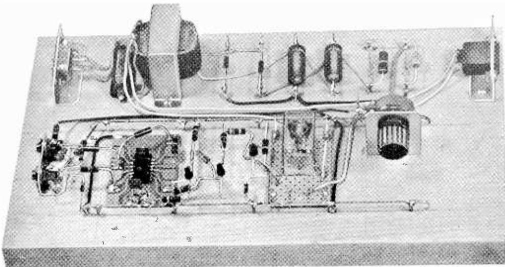
**Construction.** The circuit can be constructed on perf board or a printed circuit board. There is nothing particularly critical about the circuit. Diode  $D_4$  is mounted on the circuit board in such a way that air can circulate around it. Diode  $D_1$  is mounted outside the basement window and connected by a length of ordinary two-conductor cable. Do not place  $D_1$  where it will get direct sunlight, since the excessive heating will produce false results.
