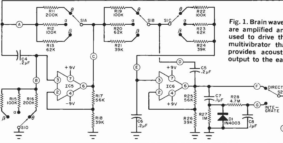
**Fig. 1. Brain waves are amplified and used to drive the multivibrator that provides acoustic output to the ear.**
