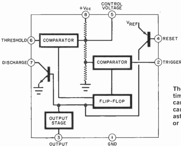
The internal circuitry of the 555 timer IC. Besides timing, the IC can be used as an oscillator and can operate in both monostable and astable modes. The output can sink or source 200 mA or drive TTL.
