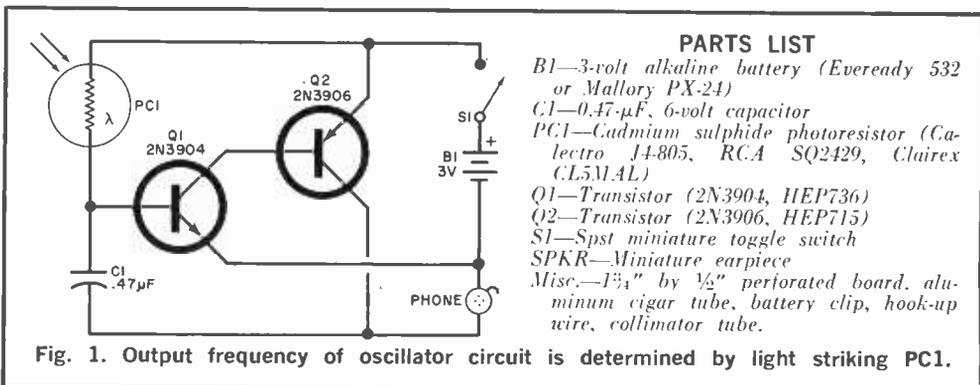
light striking the sensitive surface of a photoresistor (*PCI*). The prototype has a frequency range of up to 5500 Hz, depending on the amount of light striking *PCI*.
