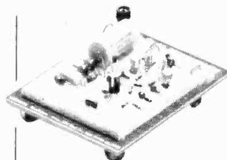
Proto Board 101. 10-14 pin DIP capacity. 5.8" long x 4.5" wide.
