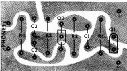
Fig. 2. PC board etching and drilling guide at top is shown full size. Directly above is component placement and orientation diagram.
