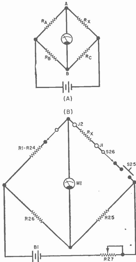
Fig. 2. The classical Wheatstone bridge is illustrated at A, while B shows how it is created in the bridge-substitution box project.
