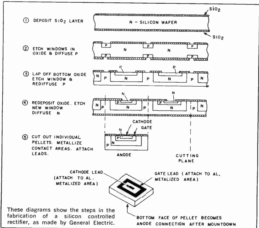
These diagrams show the steps in the fabrication of a silicon controlled rectifier, as made by General Electric.
