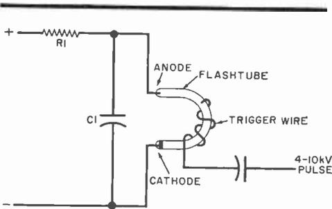
Fig. 1. In basic flash-tube circuit, C1 discharges through tube, after a trigger pulse partially ionizes gas.
