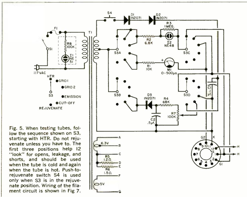
Fig. 5. When testing tubes, follow the sequence shown on S3, starting with HTR. Do not rejuvenate unless you have to. The first three positions help I2 "look" for opens, leakage, and shorts, and should be used when the tube is cold and again when the tube is hot. Push-to-rejuvenate switch S4 is used only when S3 is in the rejuvenate position. Wiring of the filament circuit is shown in Fig 7.
