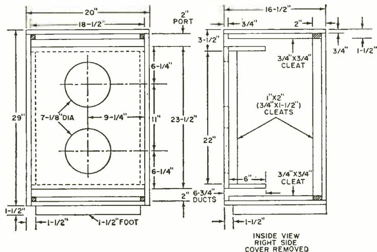
These drawings show all the necessary woodworking details. A Bill of Materials is given on page 98. Width and depth of the ports in the combined bass speaker enclosure are somewhat critical as ports are cut for the Electro-Voice speakers. The author attached poles to his column speakers so the systems could be rotated and aimed at the audience. Sound radiation from column speakers is mostly horizontal with little vertical dispersion.
