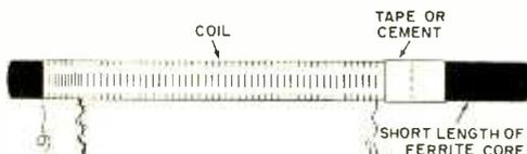
core. Simply tape or cement a short length of ferrite core to the coil end as shown; this will have the same effect as adding more turns to the coil.
