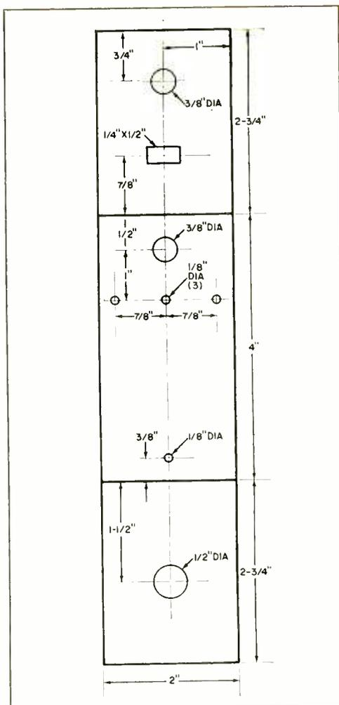
Drill holes in the outer portion of the aluminum box as shown. The size of the rectangular opening can be modified to accommodate any s.p.s.t. switch.
