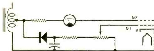
Fig. 3. Grid control is determined by the amount of negative voltage needed on G1 to obtain cutoff.
