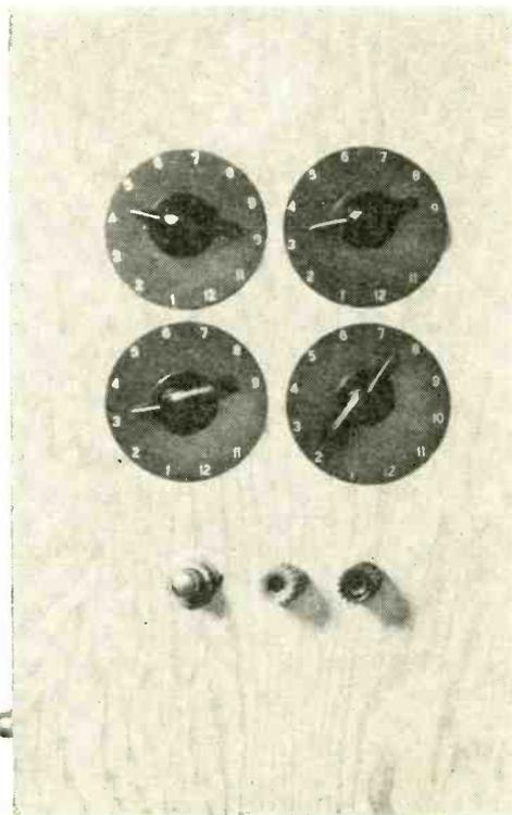
External battery can be connected to the banana jacks to overcome a weak internal battery. However, the lock cannot be opened without the combination.
