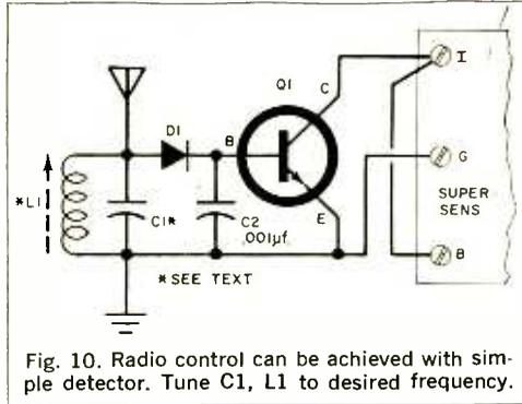
Fig. 10. Radio control can be achieved with simple detector. Tune C1, L1 to desired frequency.
