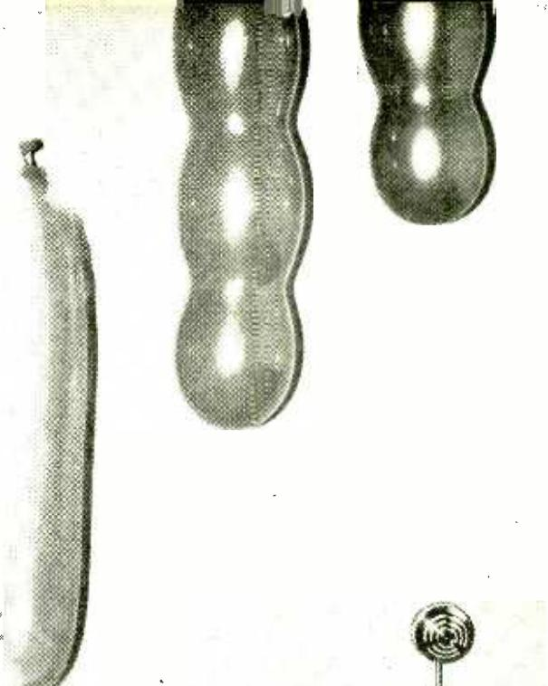
Sound-actuated unit (lower right) flashes strobe as first balloon, hit with dart, bursts. Insert shows drop of milk hitting black background; mike was 10" away, sensitivity of trip unit reduced to just half.
