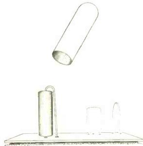
the component and the lead with a plastic "Fit-Cap," such as manufactured by the Alpha Wire Co., and apply a bit of heat. The shrinkable plastic reduces in size, grips and insulates the component.
