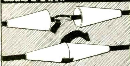
... the day Wrappington Tapely yelled "Eureka," ran into his work shop, slid a cone-shaped Mueller flexible clip insulator over each end of two wires, before splicing, then slid the insulators back together just before wrapping with tape. The high dielectric insulators not only improved insulation at the splice, but made it very easy to remove and replace the covering for inspection of the joint. What new things have you found to do, with Mueller Clips and Insulators?
