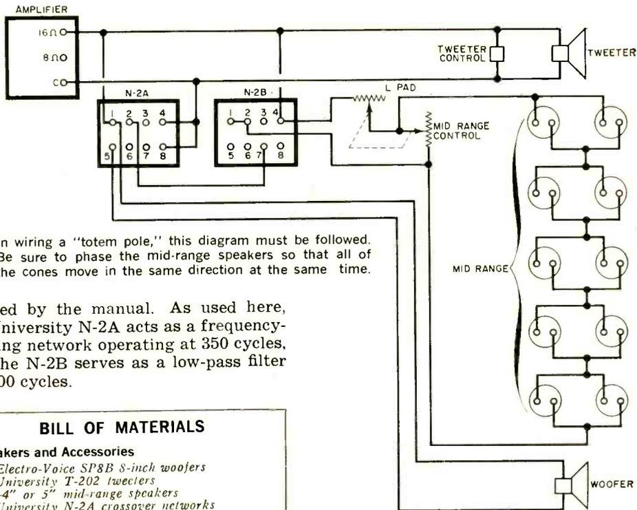
In wiring a "totem pole," this diagram must be followed. Be sure to phase the mid-range speakers so that all of the cones move in the same direction at the same time.
