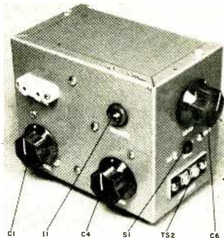
Then you can put knobs on the shafts, as shown. A large soldering iron is needed for this particular job. Don't let excess solder dribble down and short out the trimmer plates or damage the mica insulation.
