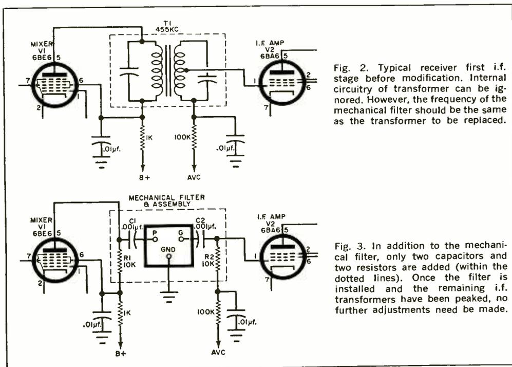
Fig. 2. Typical receiver first i.f. stage before modification. Internal circuitry of transformer can be ignored. However, the frequency of the mechanical filter should be the same as the transformer to be replaced.
