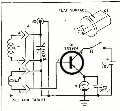
Fig. 1. Base-emitter circuit of *Q1* functions as a simple diode detector when battery is not connected; with battery, sensitivity increases tenfold.
