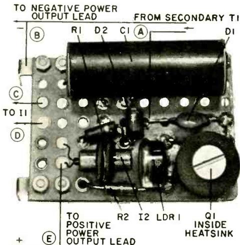
Press-fit I2 into a grommet and position the assembly close to and "facing" LDR1. A wire loop holds the grommet in place. Observe polarity of diodes.
