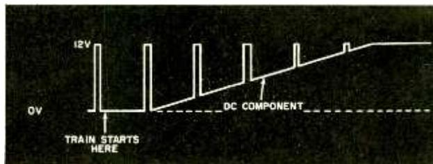
Fig. 1. The ordinary power pack is nothing more than a full-wave rectifier whose output is a pulsating d.c. voltage with peaks that look like the waveform above. For most locos, the average power required for starting is much too high for a smooth start, and the trains pull out with a sudden jerk, and at a speed not akin to real railroading.
