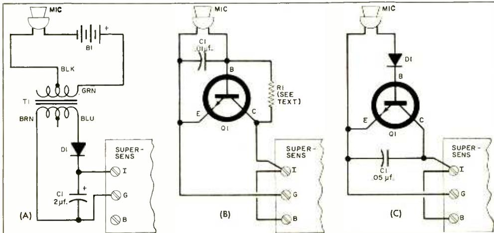
Fig. 9. Sound-actuated relays can be made. If microphone is low-impedance type, use circuit (A); high-impedance pickups work well in circuit (C); a low- or high-impedance unit can be used in circuit (B).
