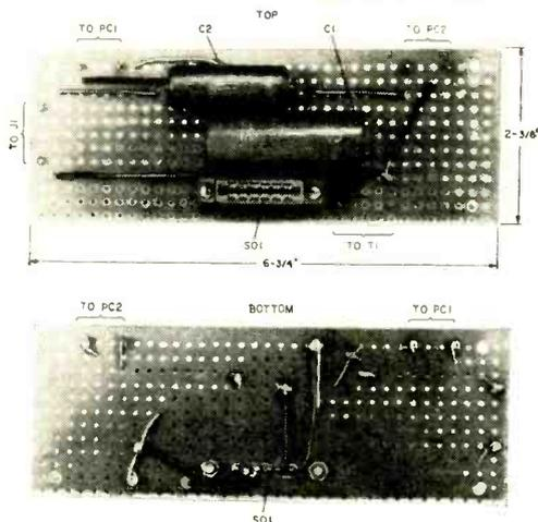
Fig. 6. Phenolic board showing components mounted on one side (top) and wiring details on other side.
