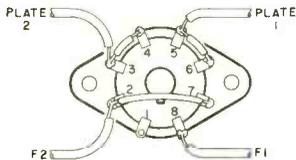
gram. Be careful not to exceed transformer and tube ratings when substituting tubes. The tubes that can be used include: the 5AR4, 5AS4, 5AT4, 5AU4, 5AW4, 5AX4, 5AZ4, 5CG4, 5R4, 5T4, 5U4, 5V3, 5V4, 5W4, 5X4, 5Y3, 5Y4, 5Z4, 5931, 6087, and 6106.
