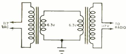
of hookup. But don't drive any equipment which requires more wattage than the lowest watt-rated winding. The transformer case and one side of the low-voltage windings can be grounded; however, the hookup will work satisfactorily without the ground connection.
