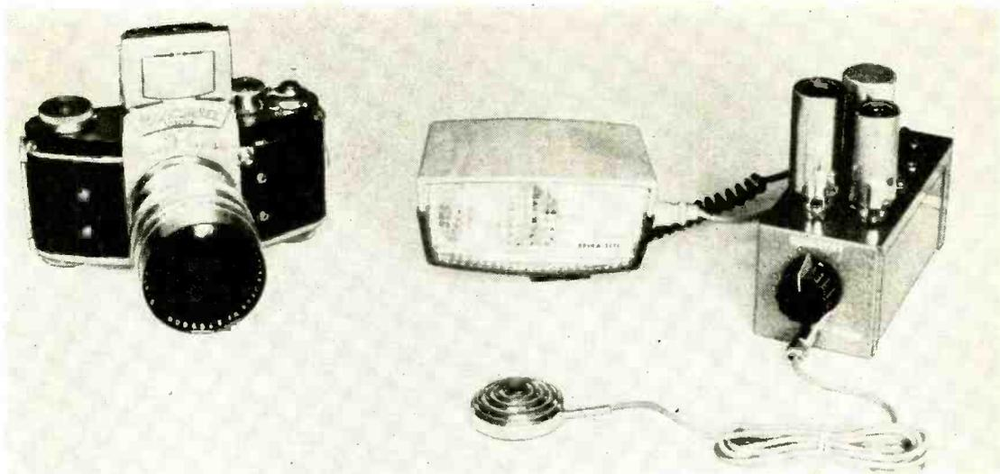
Trip unit fits neatly in  $2\frac{1}{4}'' \times 2\frac{1}{4}'' \times 5''$  box; since layout is compact, it's best to copy author's model. Strobe light is the inexpensive unit described in text.
