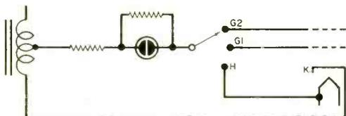
Fig. 1. Neon lamp indicator shows leakage, shorts, and opens between each element and the cathode.
