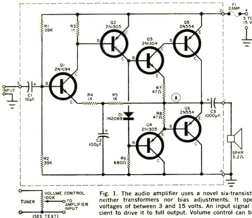
Fig. 1. The audio amplifier uses a novel six-transistor circuit requiring neither transformers nor bias adjustments. It operates with supply voltages of between 3 and 15 volts. An input signal of 0.2 volt is sufficient to drive it to full output. Volume control can be added if desired.
