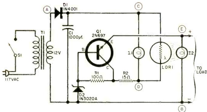
An overload indicator quickly alerts you to operating conditions. Here's what happens. Under normal load conditions the indicator light I1, protruding through the top of the cabinet, is off and the output voltage is correct. Under excessive load conditions, I1 glows and the output voltage is down sharply. When you remove the excess load, I1 will stop glowing and the output voltage will come up to normal almost instantly.
