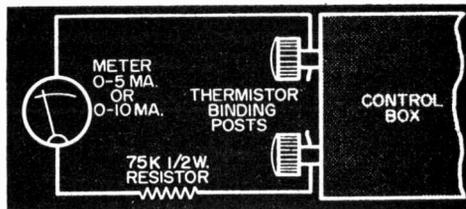
Fig. 5. Hookup for initial adjustments.
