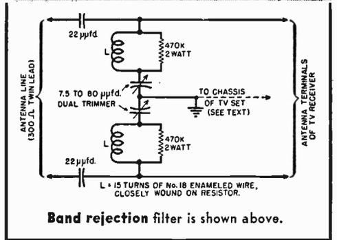
resistors is to serve as simple, inexpensive coil forms. Any style of capacitor can be used, except the paper tubular type. This type has some inductance at the higher TV channel frequencies.
