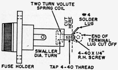
**Fig. 3. The modification of the fuse holder.**
