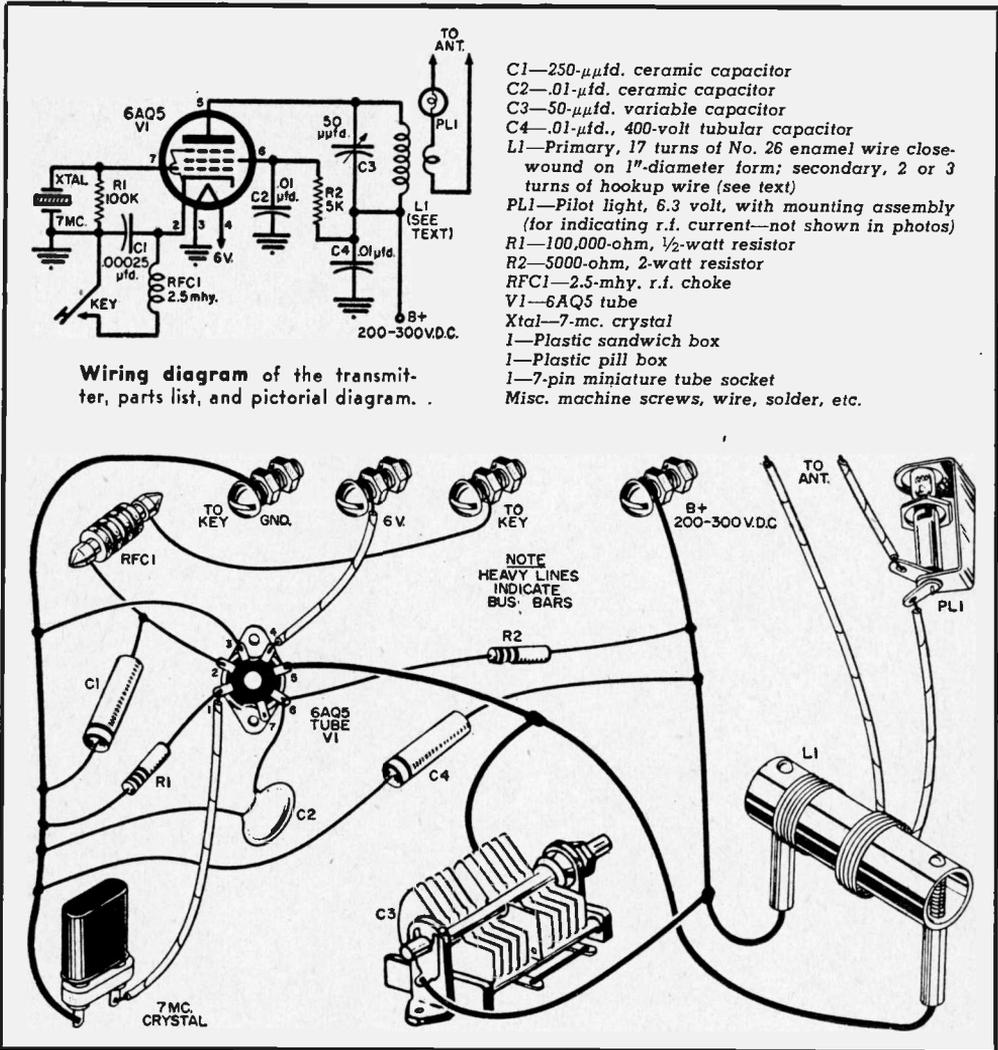
**Wiring diagram of the transmitter, parts list, and pictorial diagram.**
