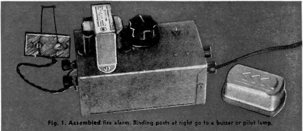
**Fig. 1. Assembled fire alarm. Binding posts at right go to a buzzer or pilot lamp.**
