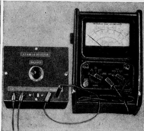
**Front panel view of the lie detector.** Any one of the readily available v.t.v.m. units may be used. The common 1000 or 20,000 ohms-per-volt meter will not permit efficient operation of the detector.
