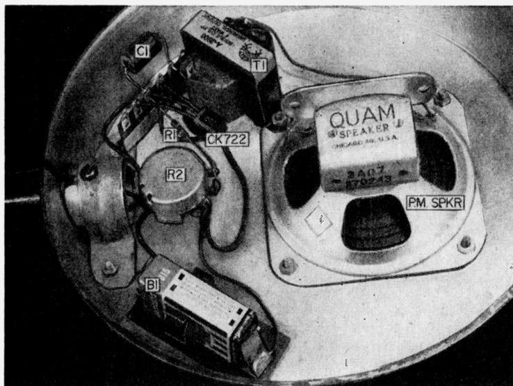
Interior view of banjo with various components identified and their relative positions indicated. The chassis is an aluminum cake pan, which contains the on-off switch S1.
