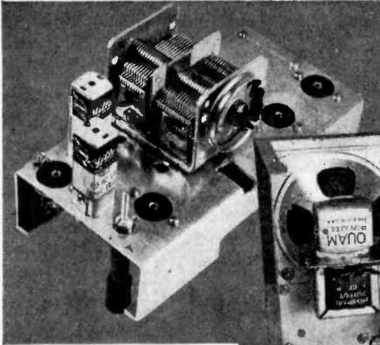
**Fig. 7.** Interior view of → the completed receiver. Because of the roomy layout, the builder should experience no construction difficulty. Mount all parts rigidly.
