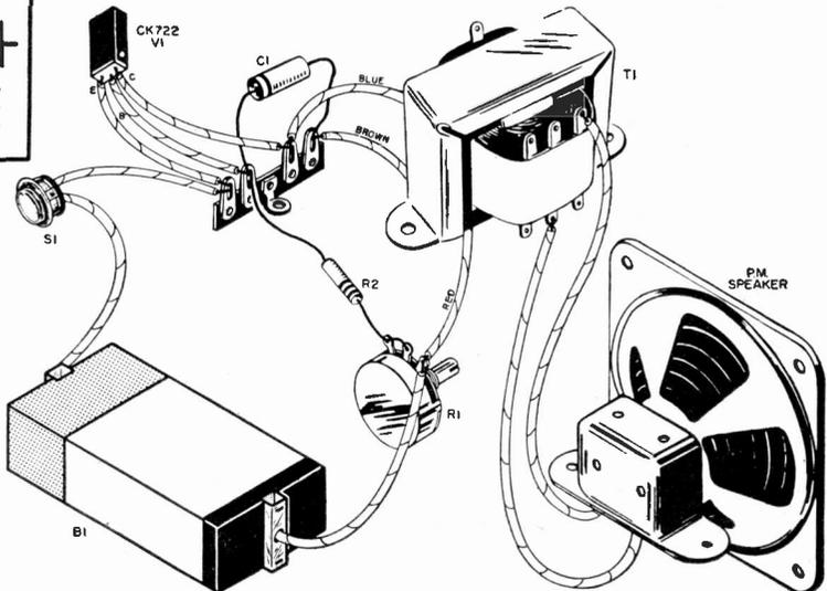
base circuits to start and sustain oscillation. The "common emitter" circuit is employed and is roughly analogous to a vacuum-tube circuit in which the emitter (E) acts as cathode, the base (B) as grid and the collector (C) as plate.
