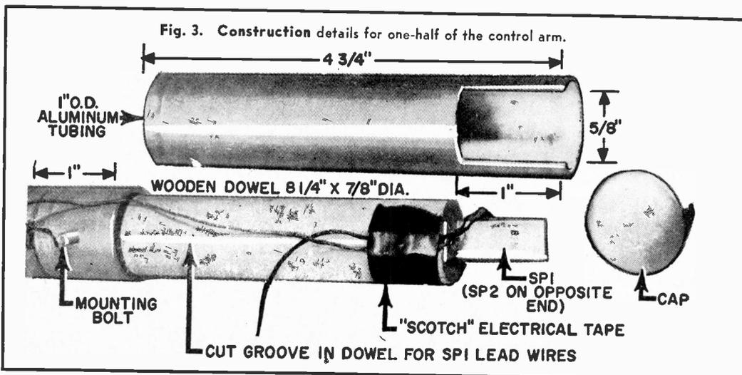
Fig. 3. Construction details for one-half of the control arm.
