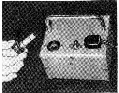
Weighing less than 2½ pounds, the first unit is housed in a 3" x 4" x 5" utility box. Fuse holder is modified to take the 1½-volt penlite cell as shown in Fig. 3 on page 76. Placing the handle off-center makes for proper mechanical balance.
