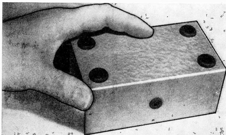
**Drill four holes** in the bottom of the metal box and insert rubber grommets to prevent scarring or scratching of furniture.
