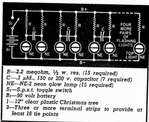
**Fig. 1. Schematic diagram and parts list covering the flashing circuit for the tree.**
