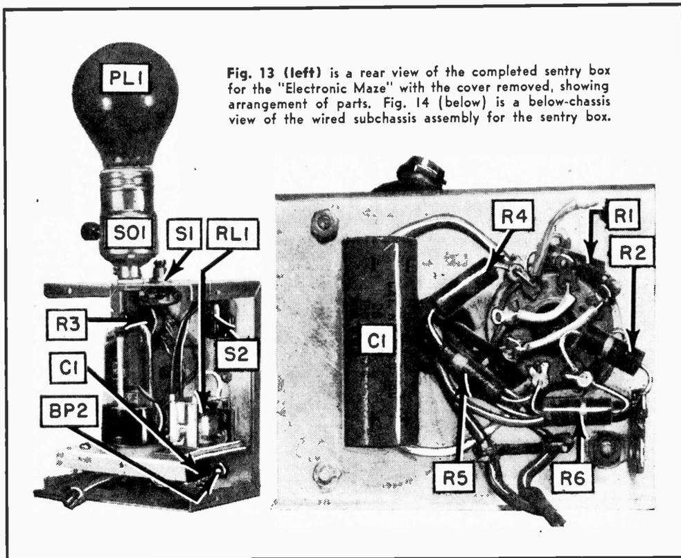
Fig. 13 (left) is a rear view of the completed sentry box for the "Electronic Maze" with the cover removed, showing arrangement of parts. Fig. 14 (below) is a below-chassis view of the wired subchassis assembly for the sentry box.
