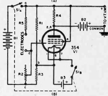
Above. Fig. 1. Schematic diagram and parts list of home-built lie detector. (A) is a simplified diagram of (B) indicating the resistance bridge.
