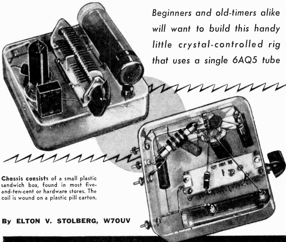
*Beginners and old-timers alike will want to build this handy little crystal-controlled rig that uses a single 6AQ5 tube*
