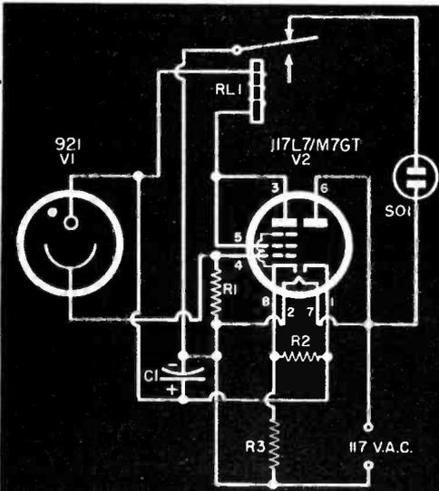
In wiring the switch, use the schematic with the pictorial wiring diagram. Note that none of the components are connected to chassis.
