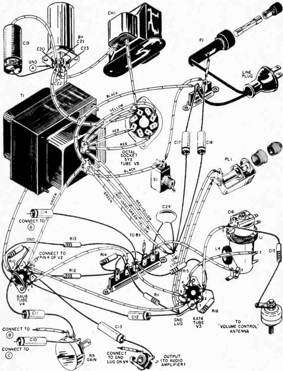
T1—Power transformer (240-0-240 v. @ 50 ma., 5 v. @ 2 a., 6.3 v. @ 2.6 a. Merit P-2958)
