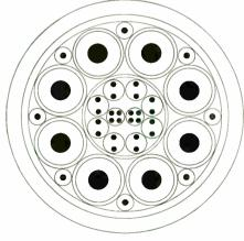
FIG. 14. NEWEST TYPE COAXIAL CABLE
