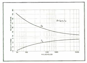
FIG. 6. IMPEDANCE CHARACTERISTICS AS A FUNCTION OF FRE-QUENCY FOR A 5-MILE LENGTH OF INSTALLED COAXIAL CABLE
