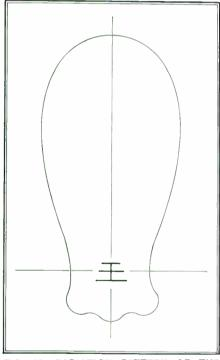
FIG. 16. RADIATION PATTERN OF THE HORIZONTAL REFLECTOR-DIRECTOR
