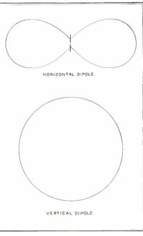
FIG. 2. RADIATION PATTERNS OF VERTICAL AND HORIZONTAL DIPOLE ANTENNAS
