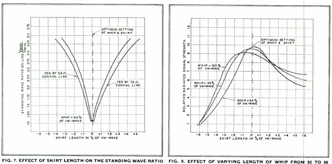
OF A SERIES-FED COAXIAL ANTENNA
