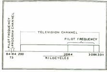
FIG. 13. ALLOCATION OF PILOT, PROGRAM, AND TELEVISION FREQUENCY CHANNELS
