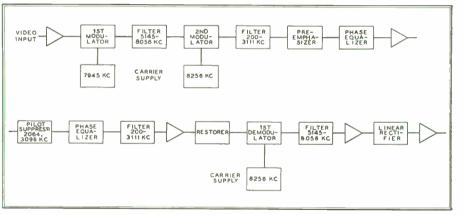
FIG. 12. BLOCK DIAGRAM OF THE TRANSMITTING AND RECEIVING TERMINALS
