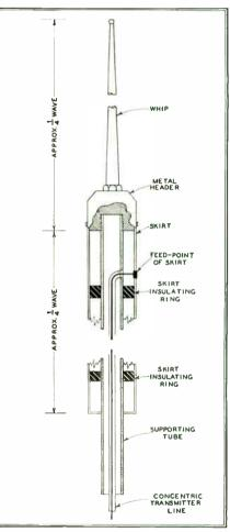
FIG. 5. SHUNT-FED TYPE OF COAXIAL, VERTICALLY POLARIZED ANTENNA
