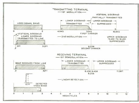
FIG. 11. MODULATION AND DEMODULATION OF SIGNALS FOR CABLE TRANSMISSION
