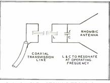
FIG. 14. SIMPLE MATCHING TRANSFORMER
