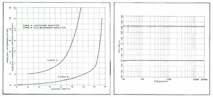
FIG. 9. COMPARISON OF INTERMODULATION WITH 2A3'S AND 6L6'S FIG. 11. FREQUENCY CHARACTERISTICS OF THE AMPLIFIER
