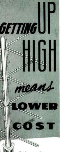
Getting that F-M Antenna up high not only means more efficient area coverage-but It also means lower costs. Doubling the height of the antenna above ground is equivalent to squaring the transmitter power. Thus, a 250 watt transmitter with a 200 foot tower would equal a 1000 watt transmitter with a 100 foot tower. That is real economy-both in initial transmitter cost and in power.
