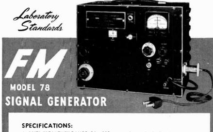
CARRIER FREQUENCY RANGE: 86 to 108 megacycles----individually calibrated dial. OUTPUT SYSTEM: 1 to 100,000 microvalts with negligible carrier leakage. OUTPUT IMPEDANCE: Constant at 17 ohms. MODULATION: 400 cycle internal audia oscillator. Deviation directly calibrated in two ranges: 0 to 30 kc. and 0 to 300 kc. Can be modulated from external audio source. Audio fidelity is flat within two db fram d.c. to 15,000 cycles. Distortion is less than 1% at 75 kc. deviatian.
