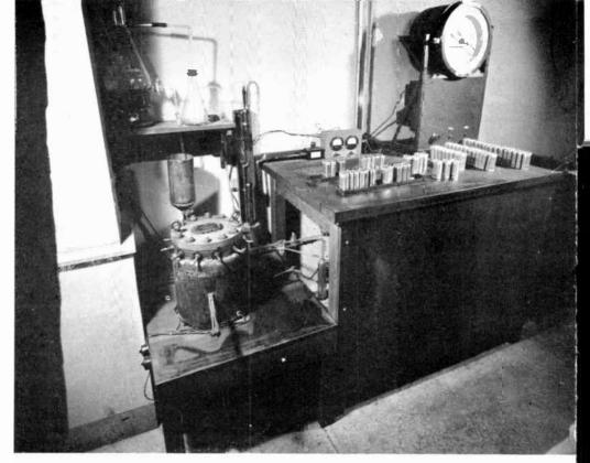
FIG. 16. A SMALL-SCALE IMPREGNATING TANK IS USED TO MANUFACTURE SAMPLE CON-DENSERS SO THAT THE CHARACTERISTICS OF THE PAPER CAN BE TESTED
