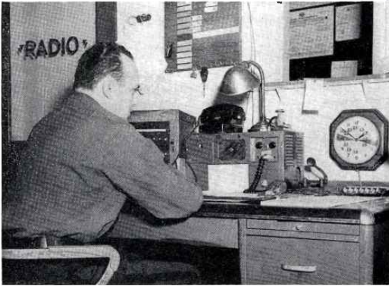
ABOVE: THE STATE POLICE HEADQUARTERS BUILDING AT BEDFORD. LEFT: THE OPERATOR'S POSITION AT THE BEDFORD BARRACKS. AN RCA VHF TRANSMITTER-RECEIVER UNIT IS INSTALLED ON THE DESK
