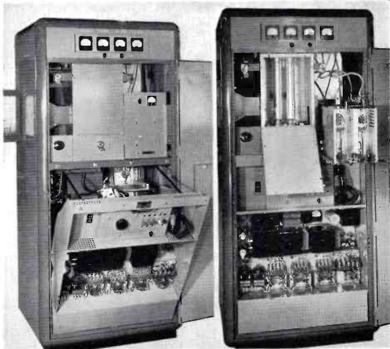
FIG. 12. QUICK ACCESS IS PROVIDED TO THE POWER SUPPLY CIRCUITS BELOW, AND TO THE SECTIONS CONTAINING THE PUSH-PULL OUTPUT TUBES AND THE INTERMEDIATE AMPLIFIER
