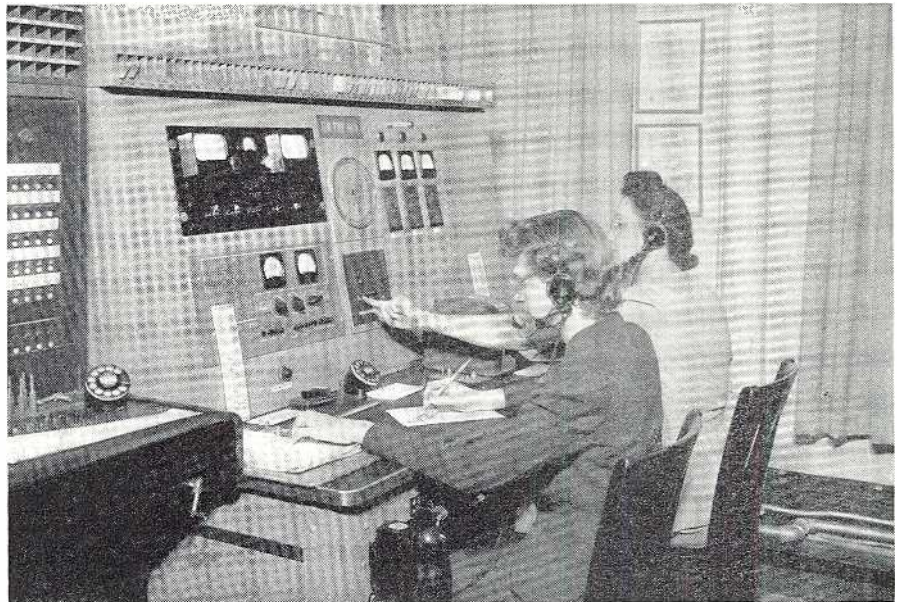
FIG. 1. TYPICAL SETUP FOR RELAYING LAND-LINE MESSAGES TO AND FROM MOBILE UNITS
