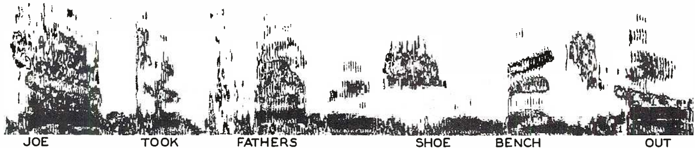
FIG. 9. EFFECT OF PLAYING ORIGINAL SAMPLE AT HALF-SPEED. FREQUENCY COMPRESSION AND ALTERATION OF ENERGY DISTRIBUTION ARE EVIDENT
