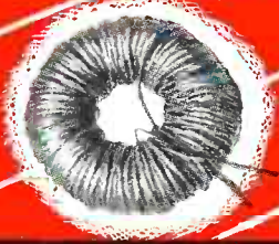
C This sub-miniature (.18 cubic inch) output transformer is intended for hearing aid and other extreme compact service. While the dimensions are only 7/16" \times 9/16" \times 3/4" , the fidelity is ample for voice frequency requirements.
