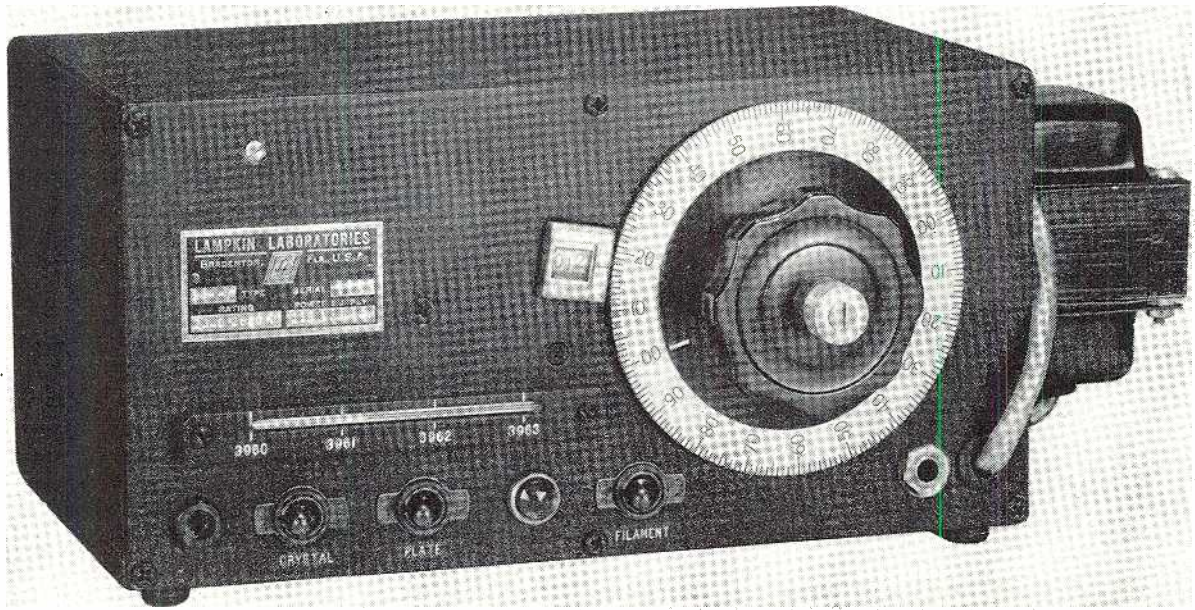
FIG. 2. THIS FREQUENCY METER HAS A THERMOMETER TO GIVE DIAL-READING CORRECTIONS FOR TEMPERATURE CHANGES AFFECTING THE CRYSTAL
