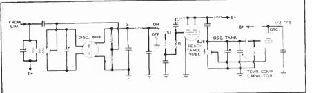
Fig. 4. Simplified diagram of AFC circuit, which employs only one additional tube
