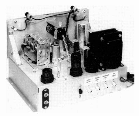
Fig. 2. Rear of model RV-10A. Note subchassis assemblies bolted to main chassis
