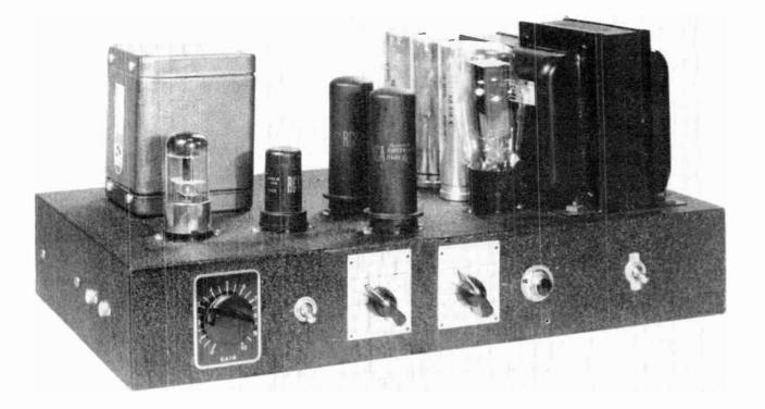
Fig. 4. Correct parts layout helps to reduce hum level. If large chassis cannot be used, power supply should be separate
