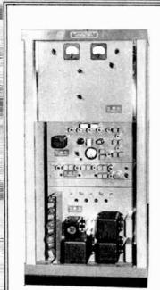
AM STATIONS CAN NOW USE REL 707-B S-T LINKS TO ELIMINATE CHARGES FOR STUDIO-TO-TRANSMITTER WIRE LINES
