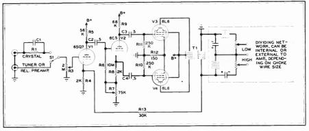
Fig. 2. Complete circuit of FAS amplifier, with one flat and one crystal input
