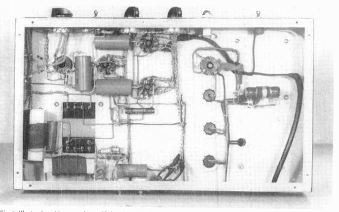
Fig. 5. Plenty of working room is provided underneath the chassis. Note extremely short AC leads from power transformer
