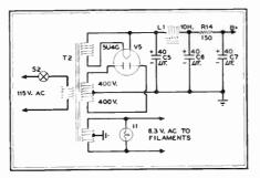
Fig. 3 Power supply has double-pi filter
