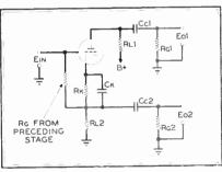
Fig. 2. Phase inversion with split load resistor
