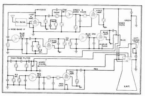
Fig. 6. Color section of simple receiver for use with frequency-interlace system October 1950—formerly FM, and FM RADIO-ELECTRONICS
