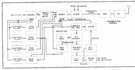
Fig. 8. Critical circuits and expensive components are located at FI transmitter
