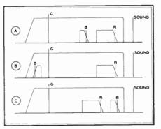
Fig. 5. Possible blue subcarrier positions
