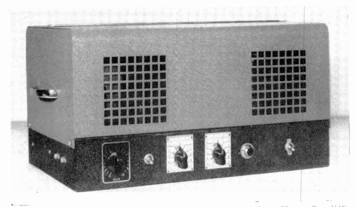
Fig. 1. The FAS amplifier, set up for demonstration purposes. Chassis-cover aids in carrying amplifier as well as shielding FM-TV, the JOURNAL of RADIO COMMUNICATION
