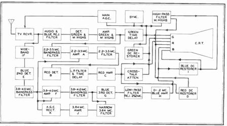
Fig. 7. Detailed diagram of a practical receiver for the frequency-interlace system
