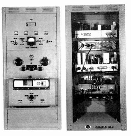
Fig. 2. Front and rear views of facsimile transmitting terminal equipment rack FM-TV, the JOURNAL of RADIO COMMUNICATION
