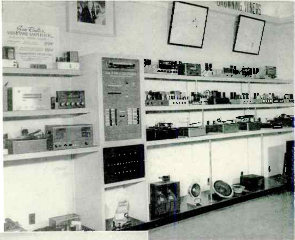
AT SUN RADIO, NEW YORK, ALL THE INSTRUMENTS DISPLAYED ARE CONNECTED TO THE CONTROL BOARD ILLUSTRATED ABOVE. PUSH-BUTTON SWITCHES SET UP ANY CIRCUIT COMBINATION TO OPERATE ANY OF THE TWELVE LOUDSPEAKERS AT THE LEFT. BELOW: SHADOWGRAPH SHOWS STYLUS MAGNIFIED 500 TIMES
