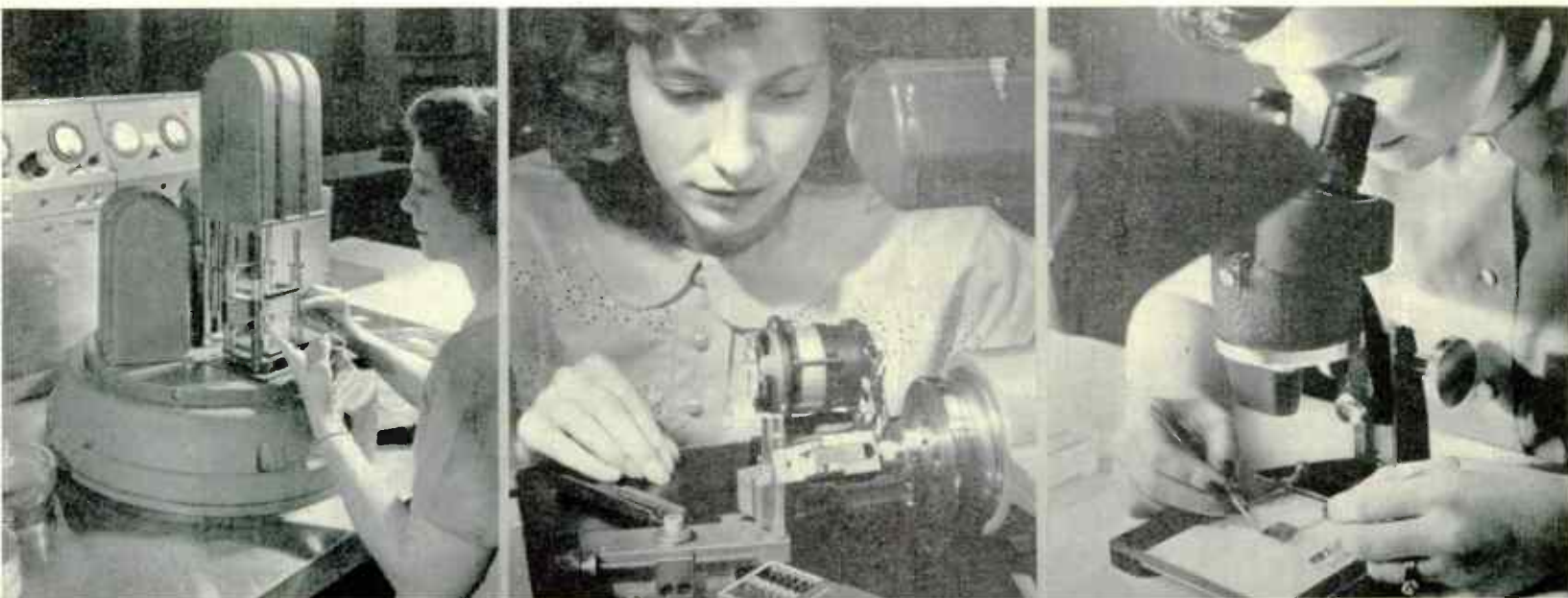
Fig. 7. Gold vapor-plating grid frames. Fig. 8. Winding grids with 3-mil tungsten wire. Fig. 9. Grids are inspected carefully
