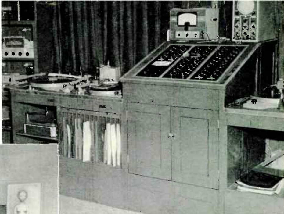
VIEWS OF THE AUDIO SETUP AT RADIO SHACK, BOSTON. ABOVE: THIS CONTROL BOARD, IN THE ROOM WHERE AUDIO EQUIPMENT IS DISPLAYED, PERMITS A-B TESTS OF RADIO-PHONO CIRCUIT COMBINATIONS. TURNTABLES AT THE LEFT ARE FOR COMPARING PICKUPS
