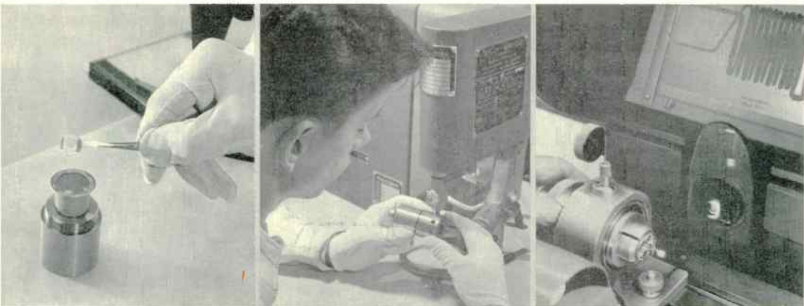
Fig. 10. Inserting finished grid. Fig. 11. Welding the retainer ring. Fig. 12. Checking heater alignment with shadow comparator
