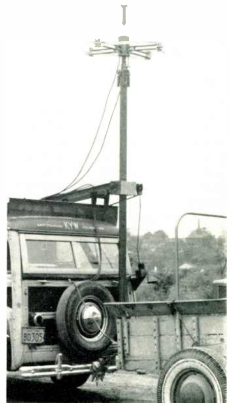
Fig. 2. Setup for mobile measurements
