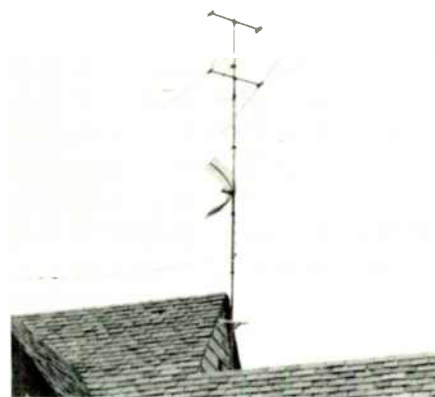
Fig. 1. UHF parabola is at mast center
