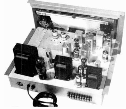
Fig. 3. Heavy steel construction and side fastening on chassis make a rugged assembly
