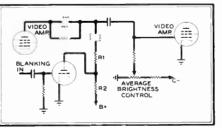
Fig. 5. A second blanking insert system
