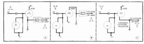
Fig. 7. Three methods of DC modulation which are used for television transmitters
