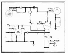
Fig. 4. Arrangement of the DC setter
