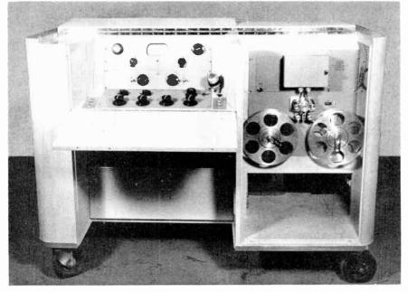
Fig. 3, Complete 35-mm, magnetic film recorder and console built into a mobile unit
