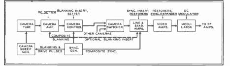
Fig. 2. Major units of a transmitter, showing the locations of the special controls
