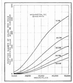
Fig. 2. Effect of rainfall on propagation
