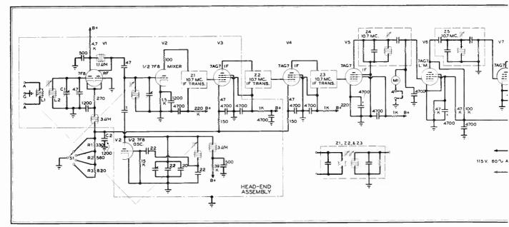
Fig. 1. Schematic of the REL model 646B receiver for the broadcast band, operating on 115 volts, 60 cycles, Model 648B is similar
