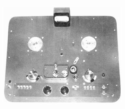
\* Engineering Department. Presto Recording Fig. 2. Layout of the tape transport system and operating controls on the top plate
