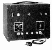
CARRIER FREQUENCIES: 4.5 Mc.; 10.7 Mc.; 21,7 Mc. (Provision for one extra frequency).
