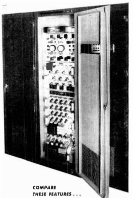
✔ Conforms to all RMA and FCC specs for standard output signals, horizontal and ver-tical driving signals, composite video blanking and synchronizing signals.
