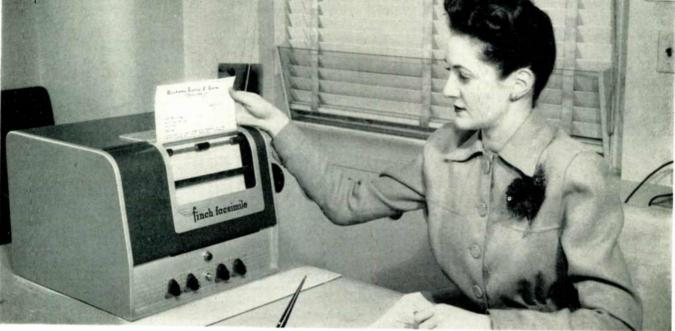
THE new Finch "Telefaxer" breaks all records for speed and accuracy in the transmission and reception of words and pictures. 30,000words per hour or 2760 sq. in. of pictures can be handled by radio. 9600 words per hour or 918 sq. in. of pictures, by ordinary telephone wire. And not one error or deviation from the original manuscript.
