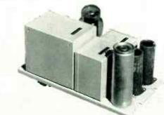
The Type 201-B Rectifier supplies plate and filament power for the Langevin Types 102, 106, 111 and similar amplifiers from a 105-125 volt, 50-60 cycle AC source. The ripple voltage of the 201-B Rectifier is 0.04% at full power output 75MA and 0.02% at a drain of 30 milliamperes.
