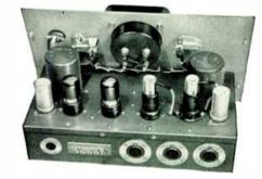
Entire chassis of both amplifiers and power supply instantly slides out of cabinets by merely urning four air lock screws on front panels. Provides complete accessibility to all components and wiring for emergency servicing. Supplied with either Cannon or Hubbell plugs.
